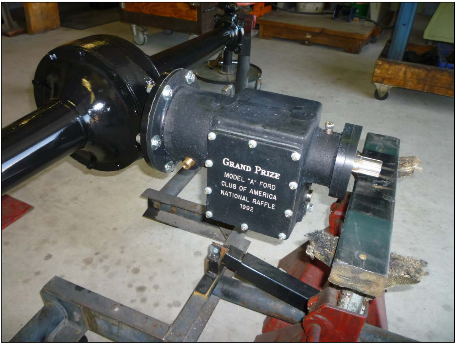
The gear housing portion of the Ryan overdrive has been attached to the banjo.
