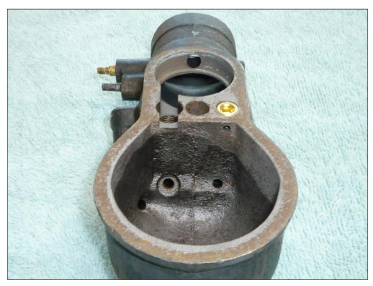
Note the slot milled into the casting right above the secondary well (threaded hole) located on the left. A hole has also been drilled into the casting in the forward area of where the venturi installs. The hole goes through to the throat of the carburetor where air is introduced. The two original vent holes on the right have been plugged off with a threaded brass plug.
