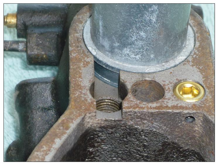
Note how the venturi with the groove machined in it accommodates the slot of the milled casting and allows air to pass around it.
