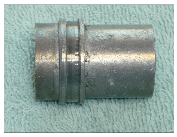
The venturi has been machined to create a groove around its circumference to allow the air coming through the drilled hole to continue to the fuel reservoir.
