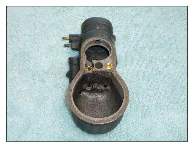
Note the secondary well installed on the left has had the top slightly milled so that the top is below the bottom of the slot milled into the casting.
