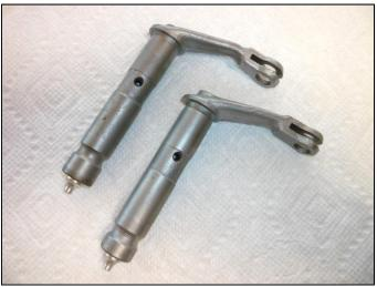
The above photo shows a pair of brake levers with grease fittings installed. Drill from the end of the shaft with a nominal  $1\8$ " drill bit down to a point between where the two bushings ride and cross drill it. Then drill the end of the shaft with a  $5\16$ " drill bit about  $3\8$ " deep.
