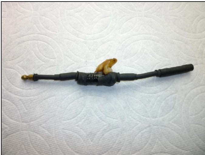
An ahooguh dropping resistor that burned out
