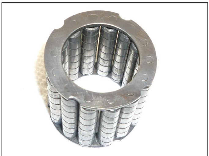
The end cap of an original roller bearing is also notched to allow grease to migrate in.
