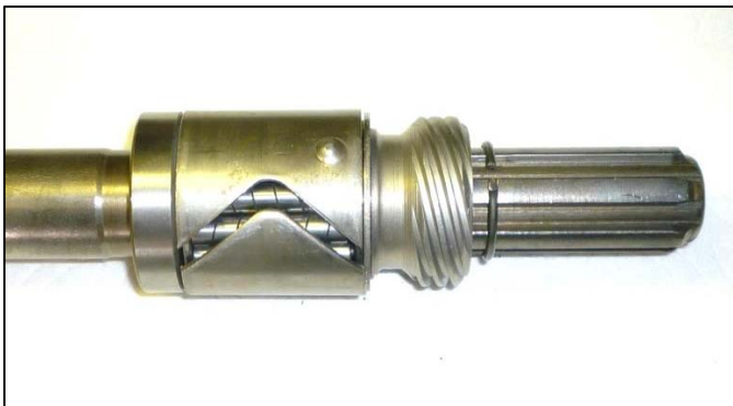
The sleeve is shown positioned around the roller bearing. Note the dimple in the sleeve.
