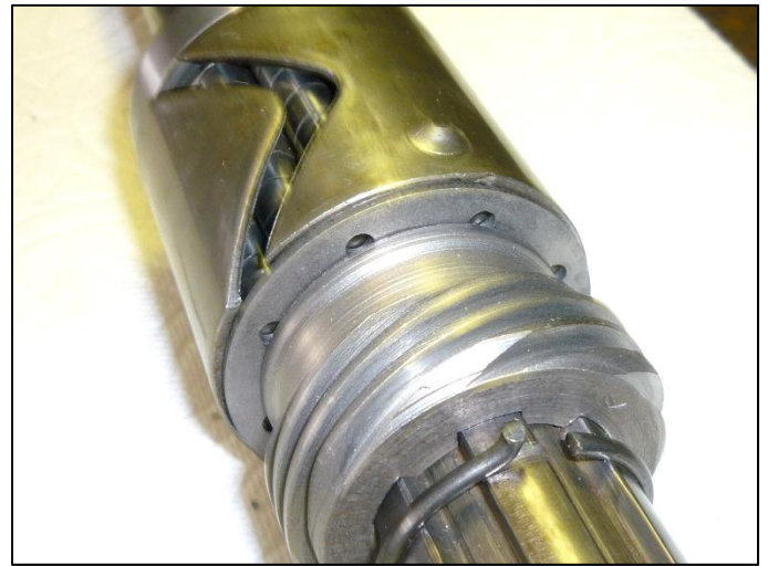
This photo shows the positioning of the thrust washer behind the speedo drive gear. The holes around the circumference allow grease pumped in the grease fitting to lube the U-joint to allow it to also flow to the roller bearing.
