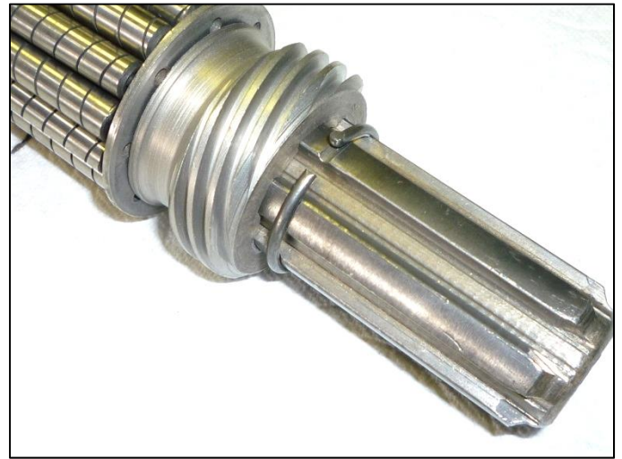
This photo shows the space between the snap ring retainer and the speedo drive gear. This nominal spacing is inherent in all Model A rear axle assemblies.
