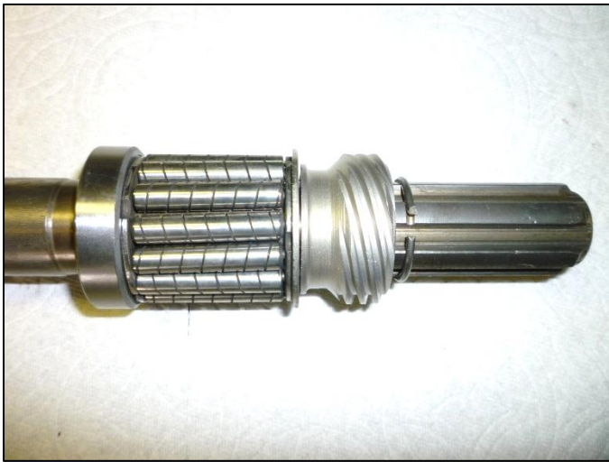
This photo shows the sequence of installed parts. From left to right the grease seal, the roller bearing, the thrust washer, the speedo drive gear, and the snap ring retainer.
