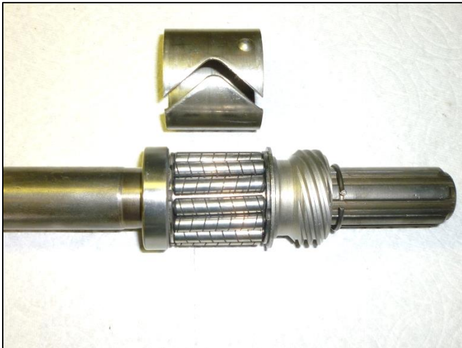
The bearing sleeve (race) is shown positioned above where it would reside in the sequence inside the torque tube.
