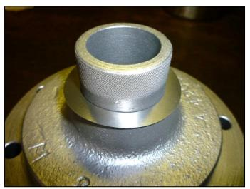
A .005 shim is installed before the new bearing is pressed on. Bratton's Antique Auto stocks the .005 shims.
