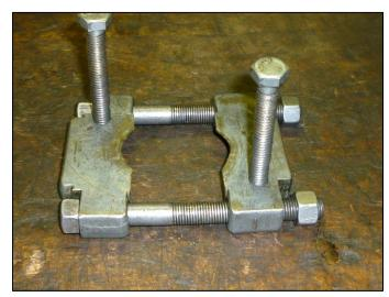
A bearing puller such as this is used to pull a bearing off of the hub without damaging the bearing. This is important if you are removing a new bearing that you intend to reinstall.
