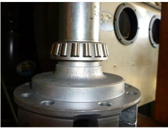
A new bearing is pressed on. The shim can be seen under the bearing. Note the second cut taken at the base of the hub will allow more room under the bearing for a bearing puller if additional shims are required.
