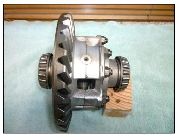
The carrier has the ring gear attached to the left side. The spider gears are inside the two carrier halves. A rear axle shaft will protrude from each side. There is a carrier bearing on each side that is mounted to the hubs with an interference press fit. The carrier bearings must be set up against their races with a pre-load of 20 inch pounds.
