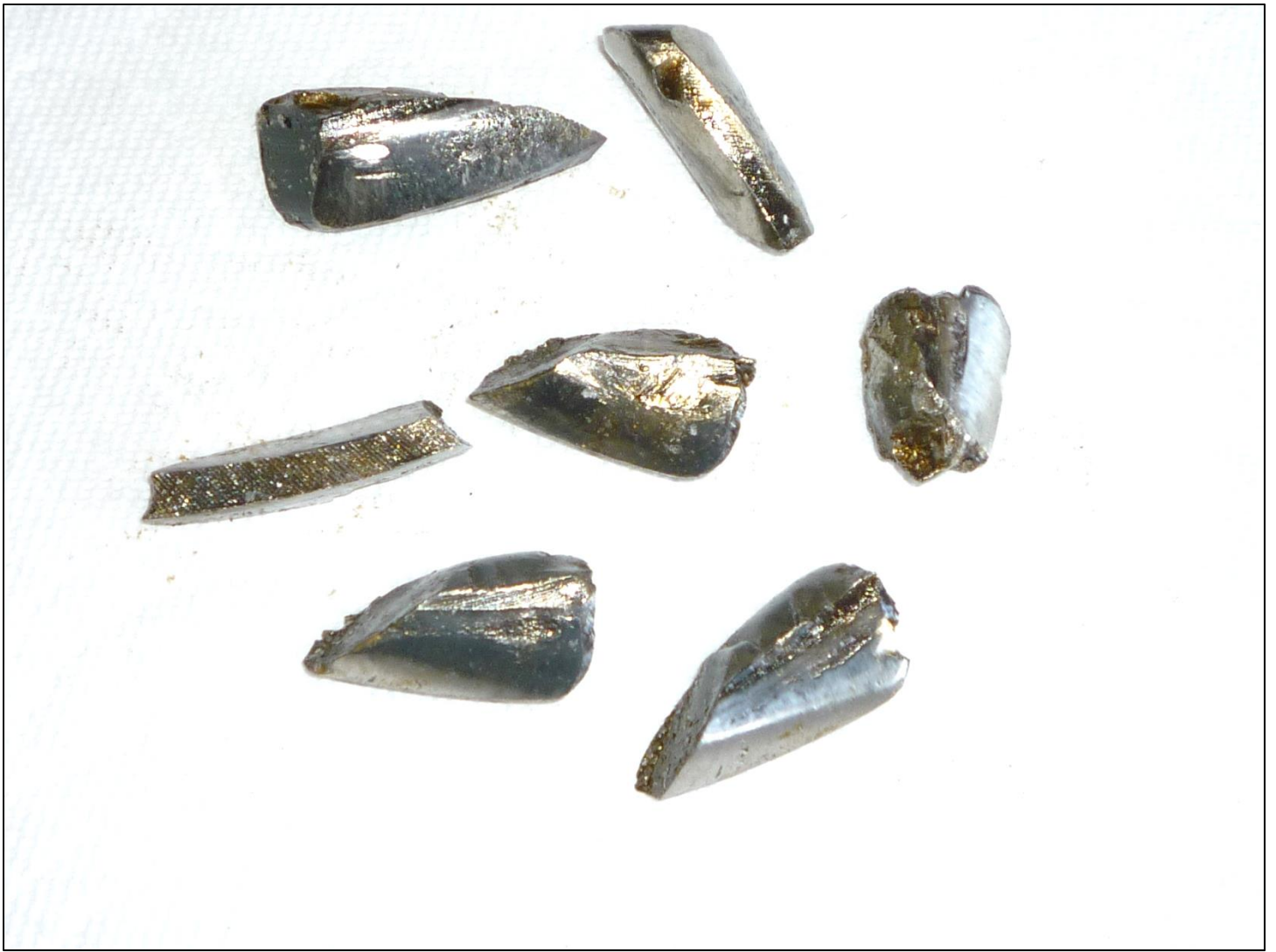
Teeth from both the ring and the pinion found lying in the bottom of the banjo.
