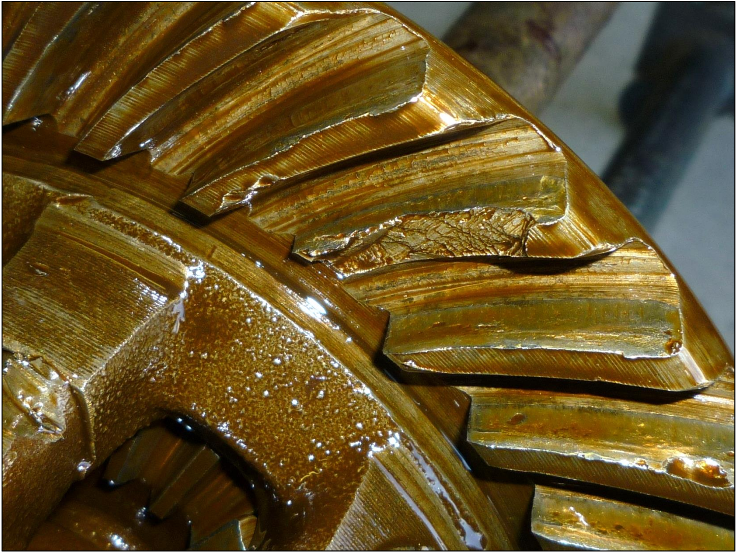
One tooth was knocked off the ring gear, along with damage to many others.
