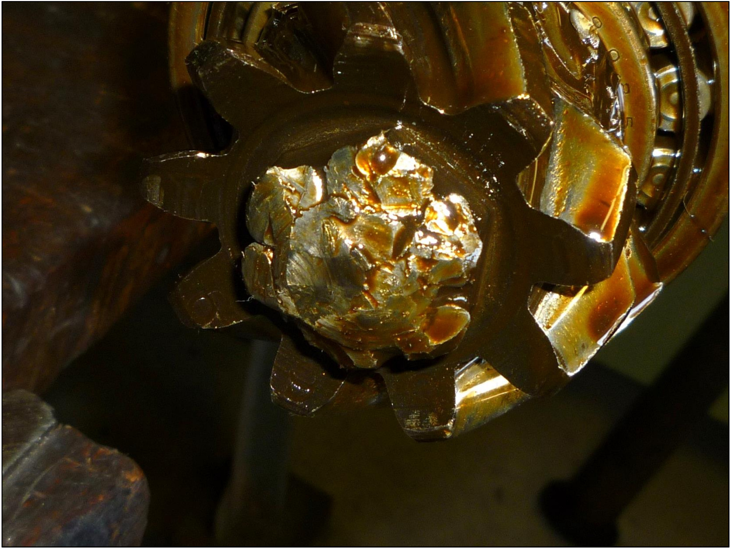
The nut on the end of the drive shaft is battered along with a number of threads on the drive shaft and the cotter pin hole.
