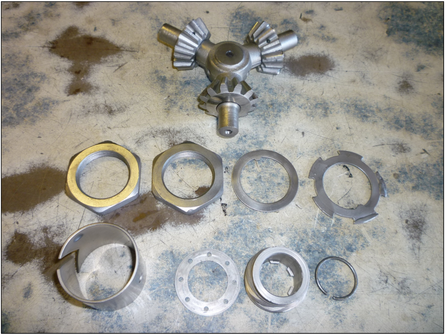
Undamaged spider gears and other hardware cleaned up and ready for installation:
