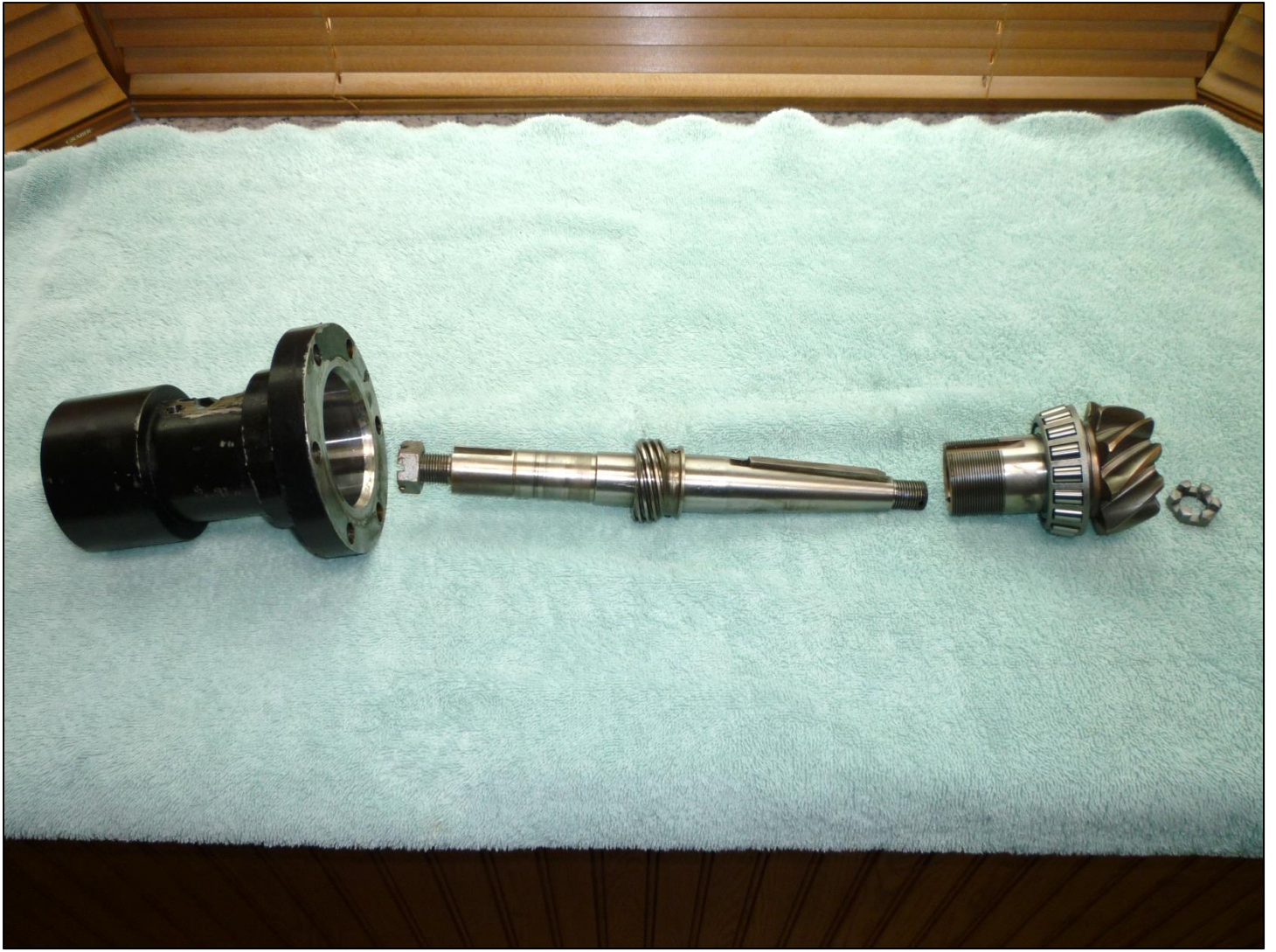
The sequence of the torque tube, drive shaft, and pinion gear:
