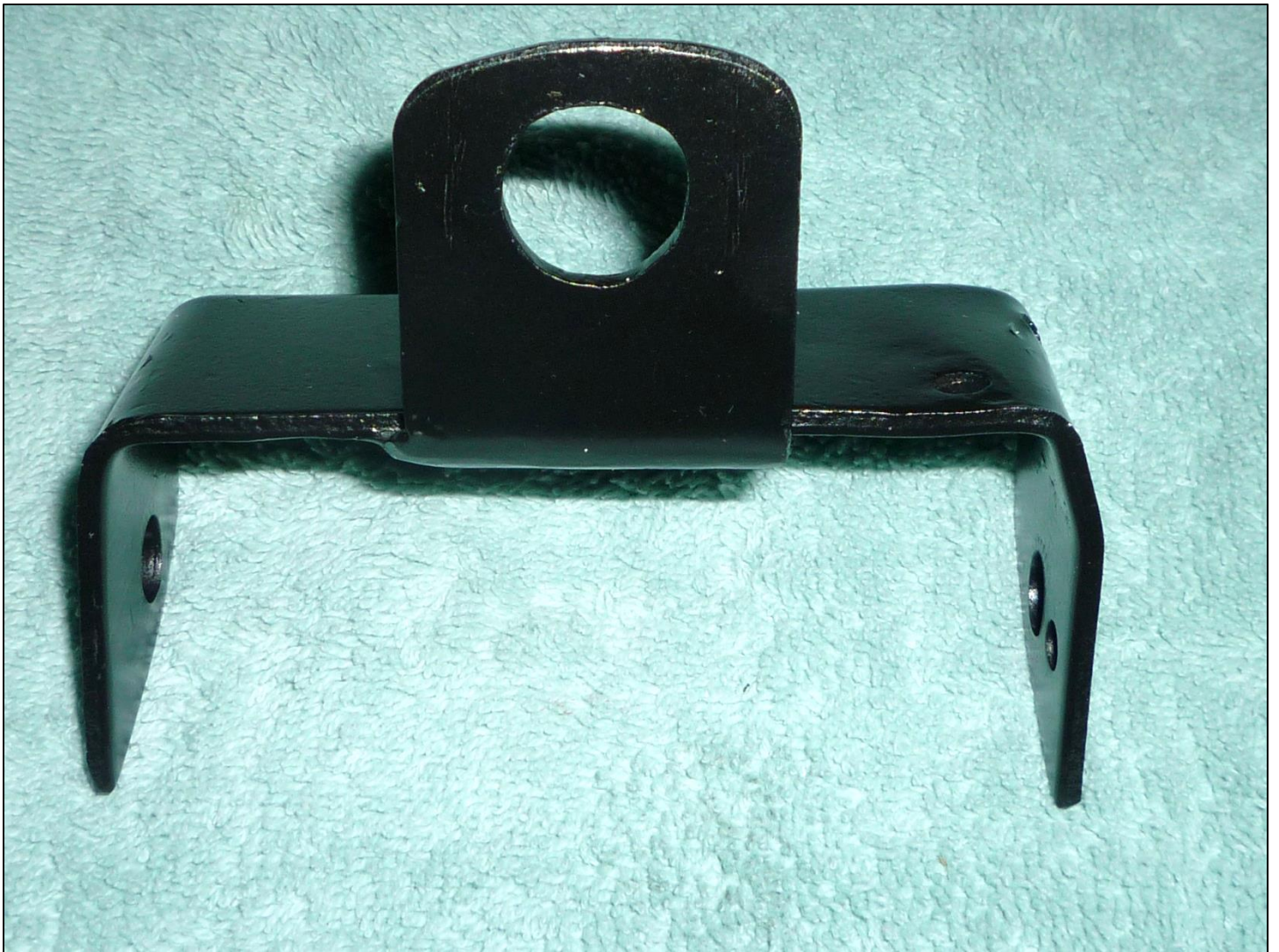
A view of the bracket that attaches to the top of the banjo to support the hydraulic brake line assembly: It has been bead blasted and painted.
