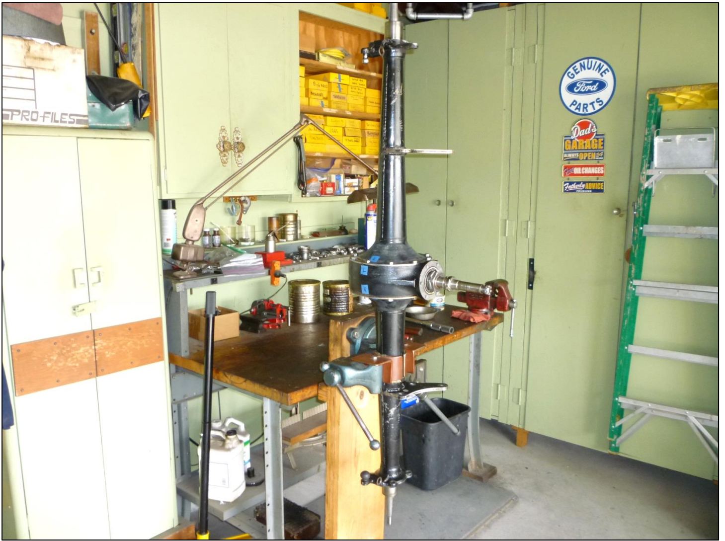
The completed rear axle assembly is shown sitting in the repair jig. The pre-loads have all been established and the carrier assembly, with both axle shafts and spider gears installed.
