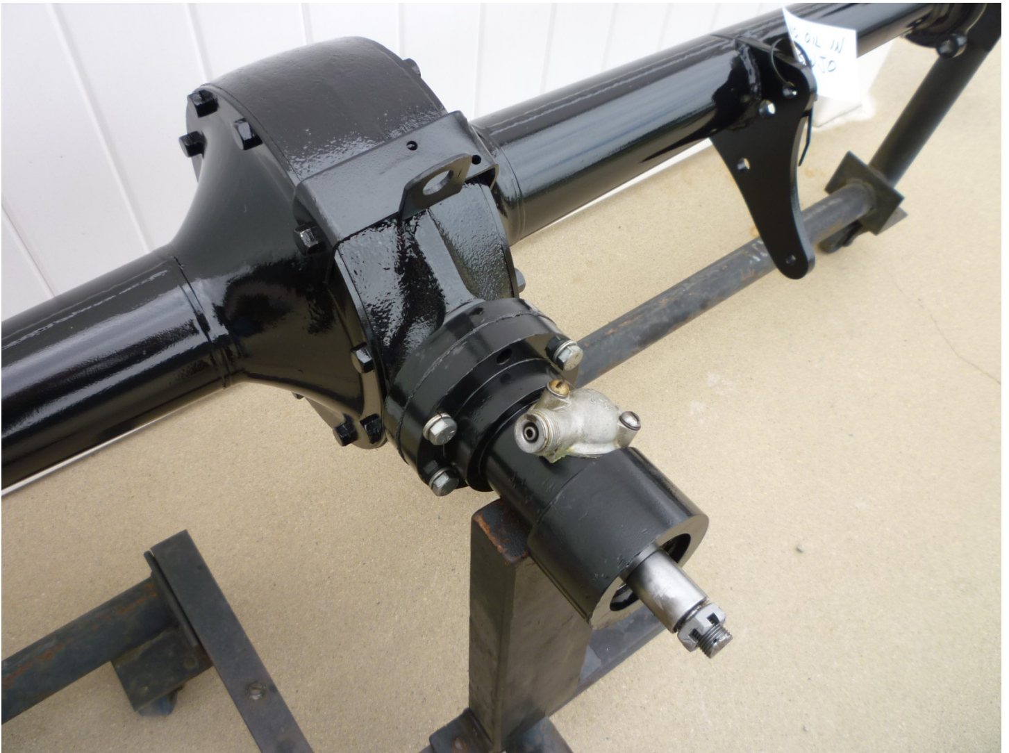
The "torque tube" and the hydraulic line support have been installed.
