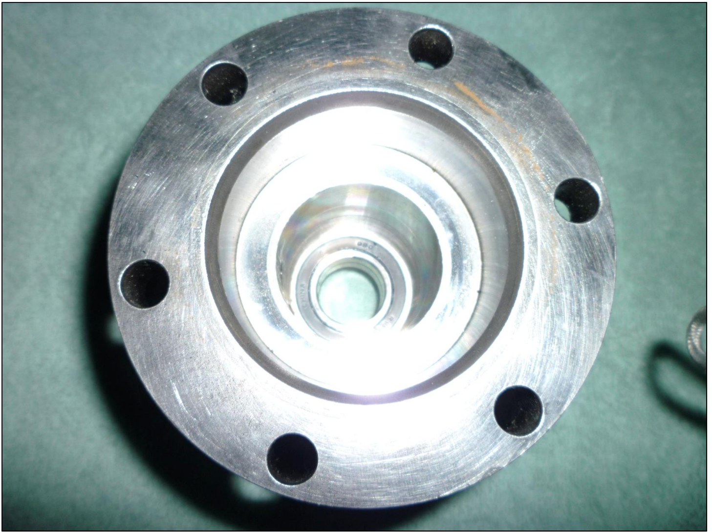
The banjo end of the torque tube housing is shown here. The two small sealed ball bearings can be seen at the bottom at the opposite end of the mounting flange.
