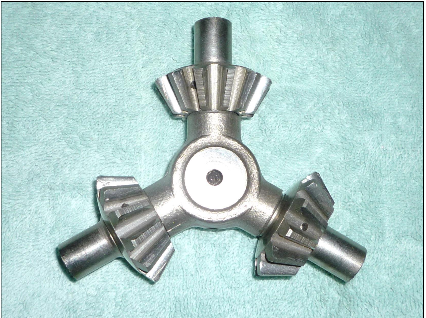
The spider gear assembly was not damaged and appears to be in excellent condition: Note the holes in each gear. This was incorporated in 1931 to provide better oiling to the three shafts on the yoke.
