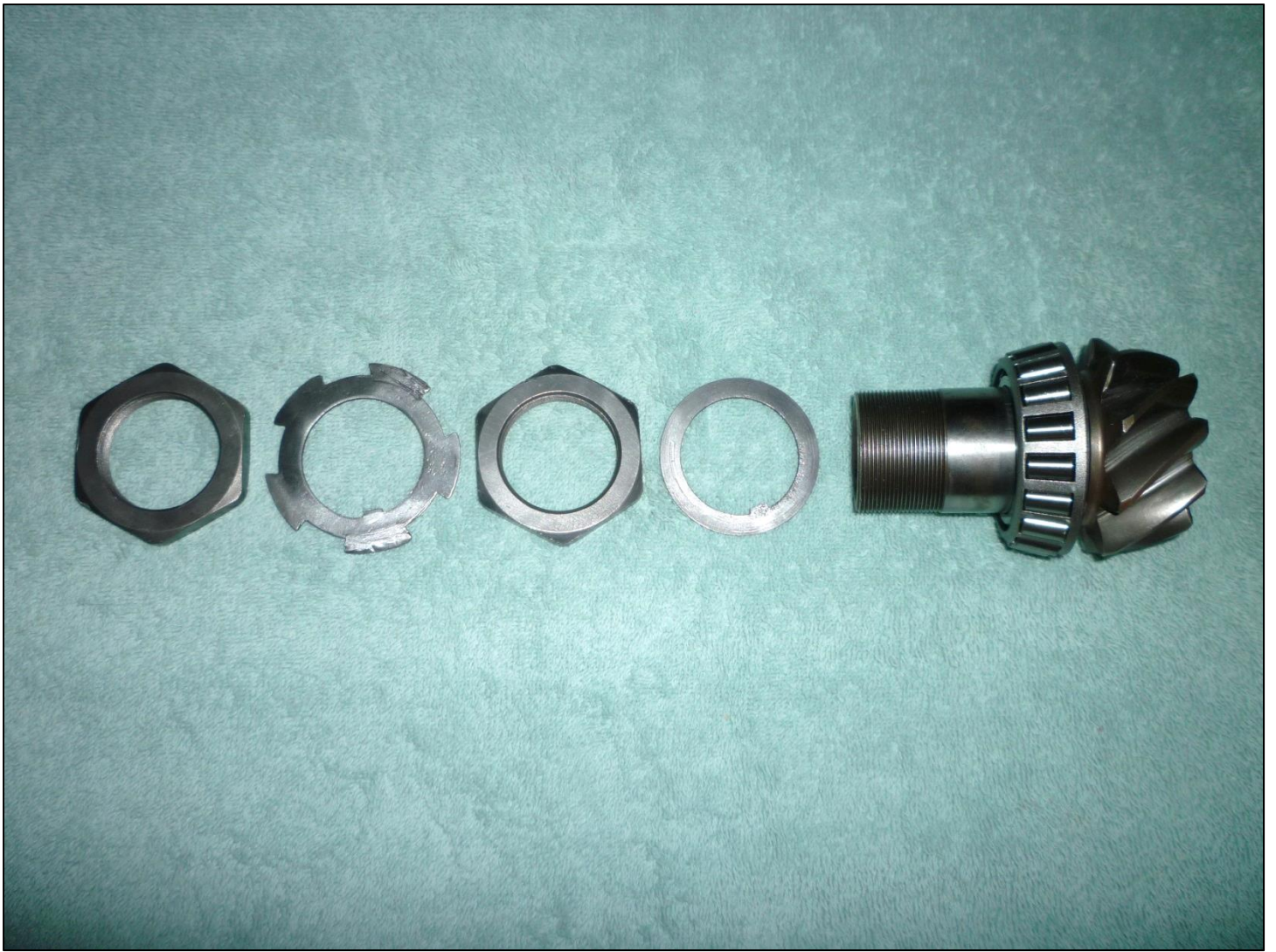
A view of the undamaged pinion gear with a new rear bearing installed:
