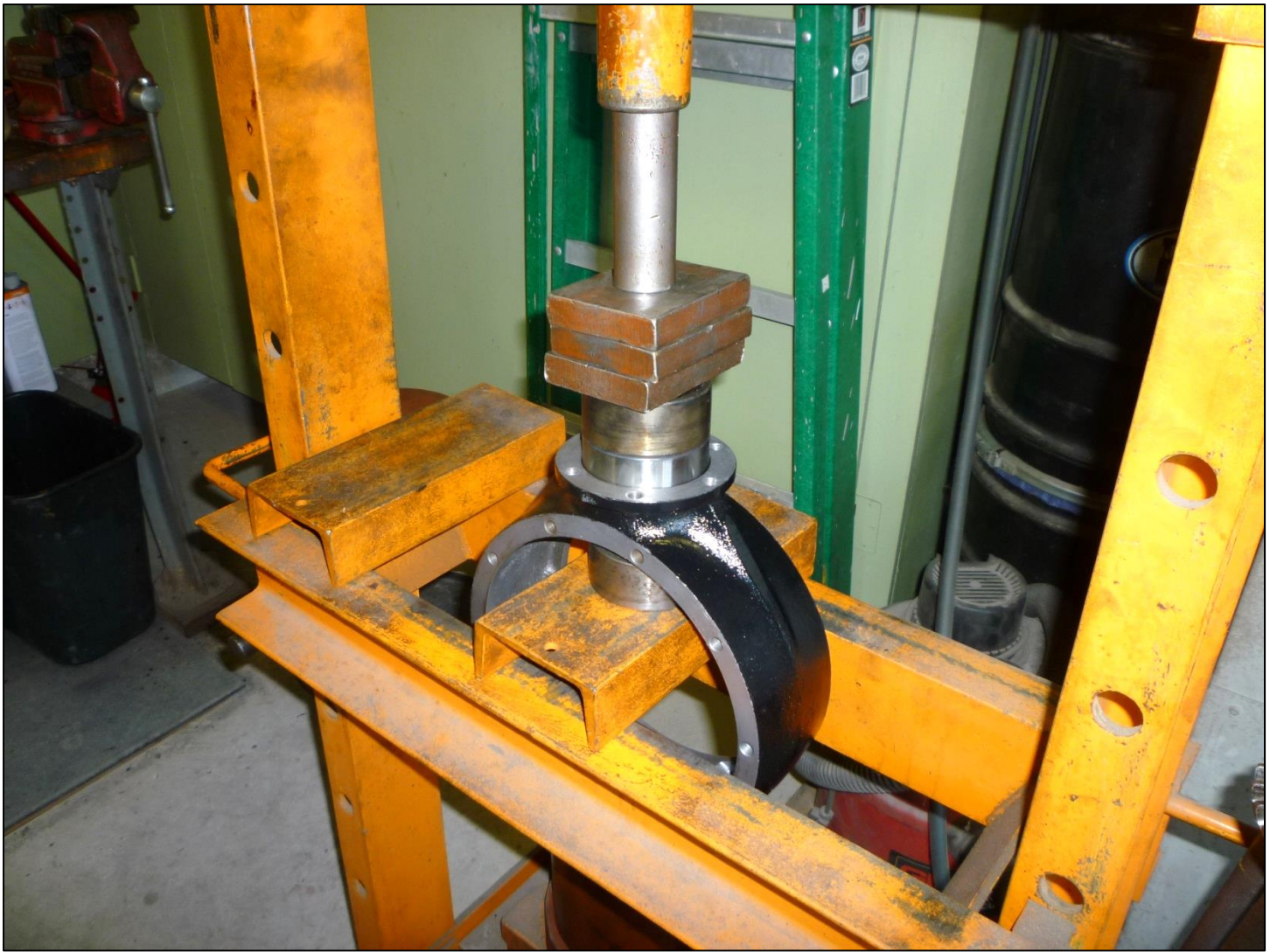
A new race is being pressed into a replacement banjo.
