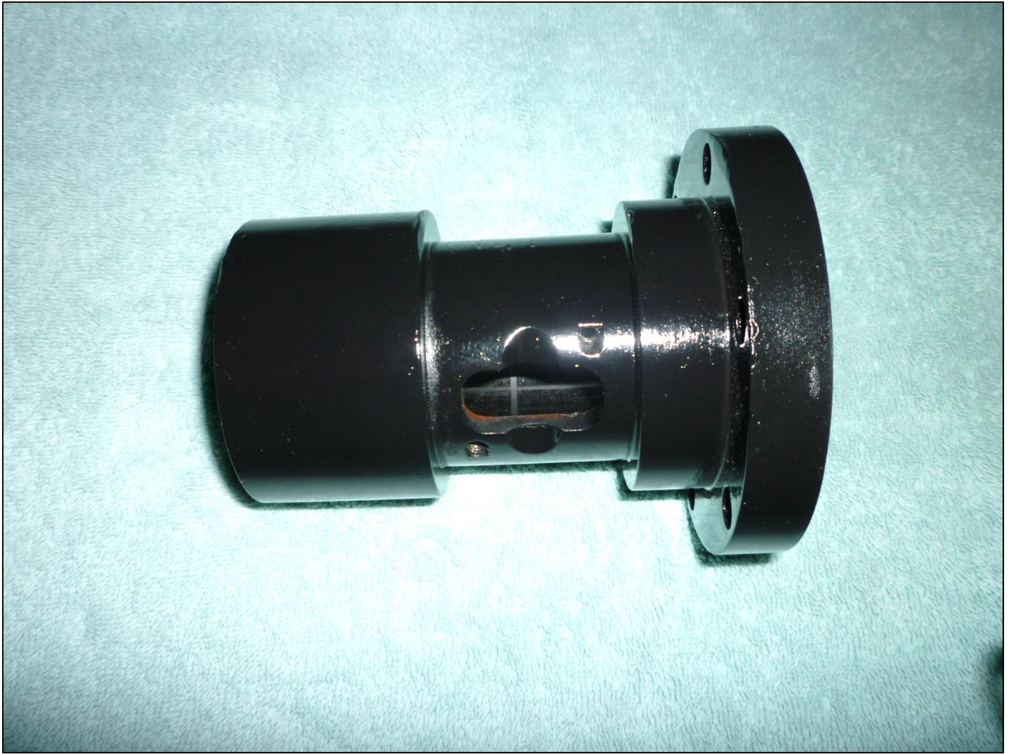
The torque tube housing has been cleaned up and painted:
