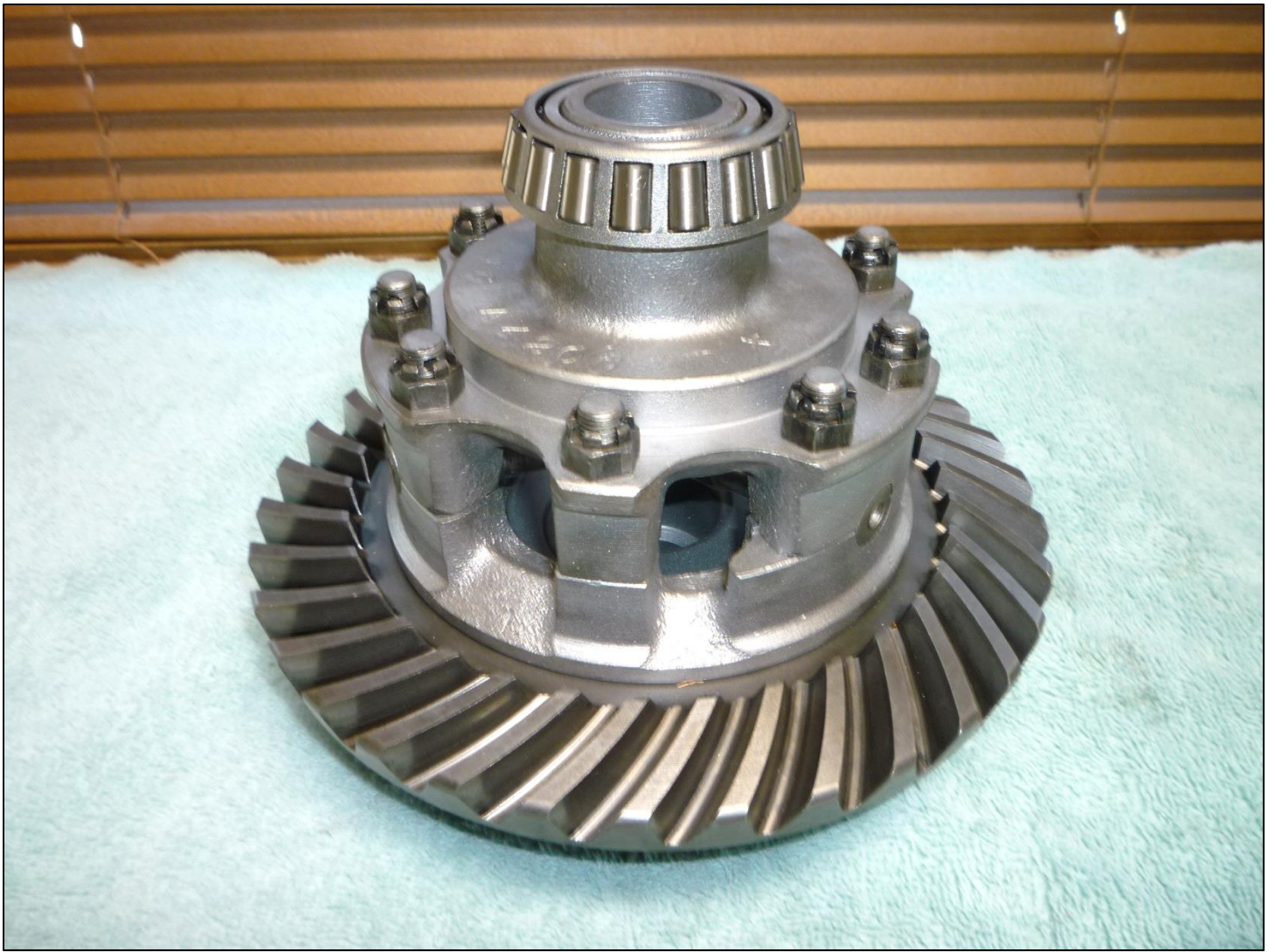
Another view of the replacement carrier and the ring gear: The ring gear was undamaged and appears to be in excellent condition.
