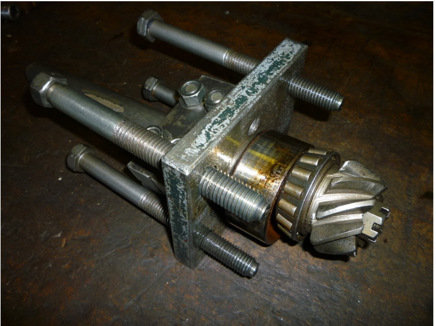
Photo shows a pinion gear assembly that has been pulled out of a banjo using the puller tool.
