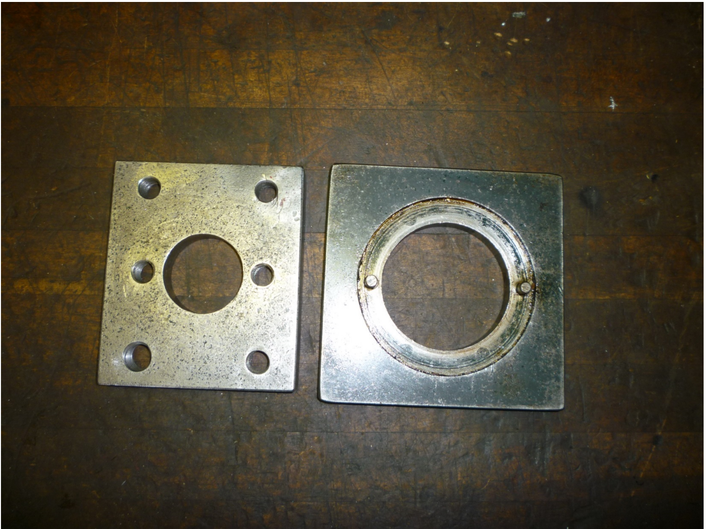
The plate on the right is mounted to the banjo flange with the two locating pins inserted top and bottom into the banjo flange bolt holes.
