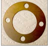
The four flywheel to crankshaft mounting bolts must be the proper length. If they are too long, they protrude through and interfere with the rear main bearing and possibly do damage to it. The retainer disk must also be installed as it affects the overall length of the bolts. Lock washers should not be used as they will position the heads of the bolts such that they will contact the springs in the clutch disk.
