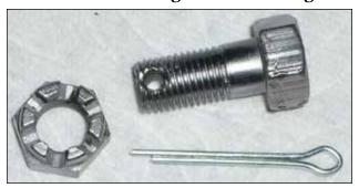
The four mounting bolts and nuts used on each front wheel backing plate must be oriented correctly with the nuts on the outside facing the center of the car. This then orients the heads of the bolts on the inside of the brake drum. This is exactly opposite to how the rear backing plates are mounted, which causes confusion. Quite often the front bolts are found oriented incorrectly. This causes the rotating hardware inside the drum to contact the edges of the castle nuts.
