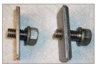
A change was made in the machining of the cluster gear shaft in the manner in which it is retained at the rear of the transmission housing. The early shafts were retained with a 3/16 inch-thick retaining plate described as a retainer for the counter and reverse idler shafts. The length of the bolt used was one inch long.
