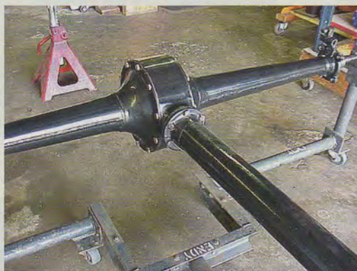
#2. Close up view. The torque tube is to be removed by removing the safety wire and the six mounting bolts. Remove the speedometer drive assembly and the snap ring in front of the speedometer drive gear before pulling the torque tube off. The torque tube, drive shaft, and the speedometer drive gear assembly will not be used with the overdrive. Speedometer operation will be obtained at the output gear of the overdrive. An extension speedometer cable is supplied with the Mitchell overdrive that will connect to the existing speedometer cable.
