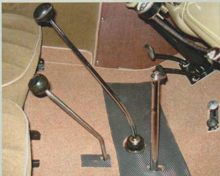
#23. The Mitchell shifter is located behind and to the right of the standard shifter. Shift it forward and you are in overdrive. Shift it backwards and you are out of overdrive. The overdrive can be used in any gear and is particularly beneficial in second gear-overdrive when driving in mountainous terrain.
