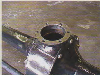
#9. Close up view of the banjo with pinion removed. Oil in the banjo does not have to be drained.
