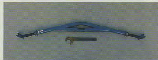
A suitable and safe spring spreader.
