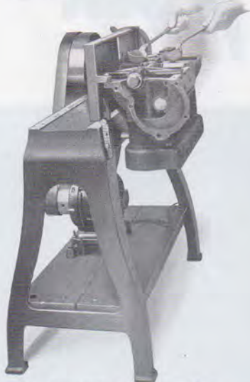
Position Of The Block Makes Pouring Easy.
