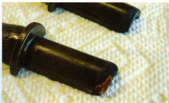
The rusted tip of the valve guide from the exhaust port of the number two cylinder.
