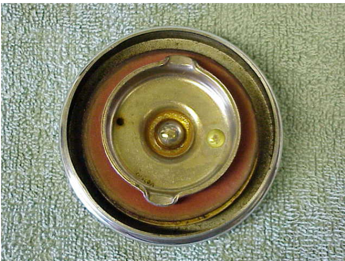
Modified gas cap with a small rivet epoxyed into place opposite from the vent hole.
