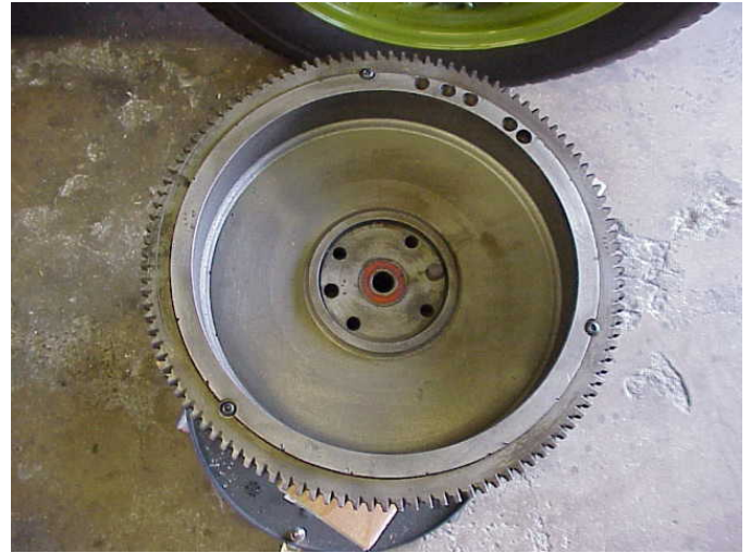
Three setscrews are installed at 120 degrees distance from each other.
