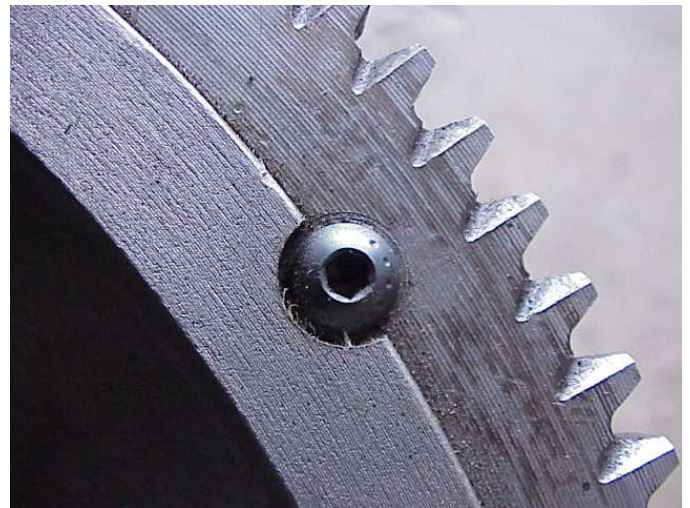
The setscrews lock the ring gear to the flywheel.
