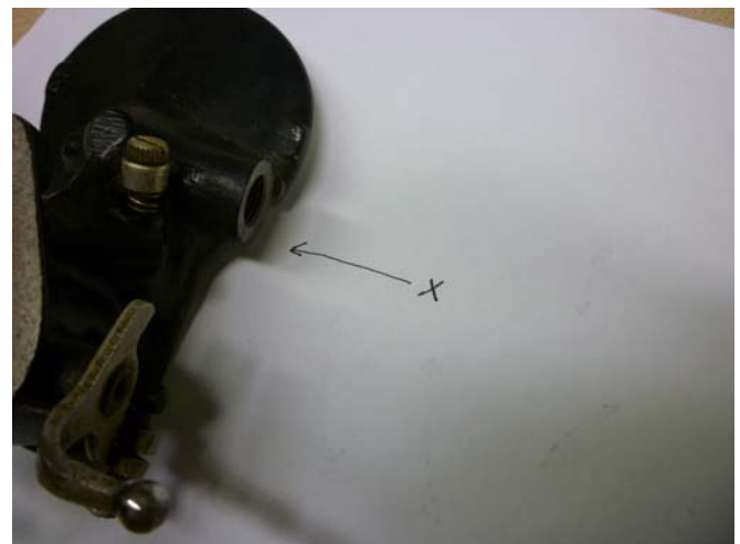
Side bowl carburetor top casting
