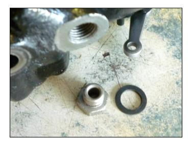
There is an easy repair. Salvage a filter screen assembly from a top casting. Unsolder the screen from the hex. The hex is cup shaped as is the original drain boss plug to act as a small fuel reservoir. The difference is the original drain boss plug has a 1/2" hex and the filter screen has a 5/8" hex and larger threads.
