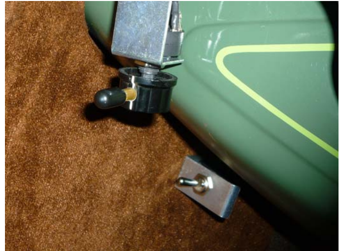
The turn signal switch is mounted under the left side of the dash rail. The emergency flasher is mounted to the left kick panel.
