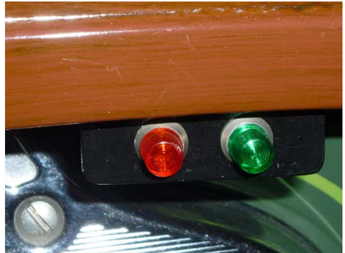
An added feature to the installation was the inclusion of two very small signal lights mounted on a bracket that just peeks out from under the dash rail. The light on the left is red; the light on the right is green. They flash in concert with whichever signal lights are flashing.
