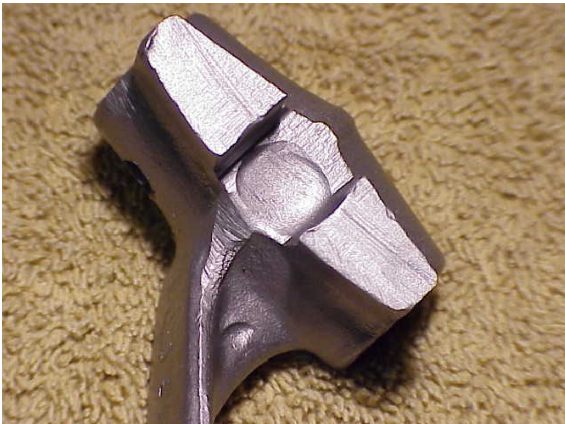
Trans tower fork worn
