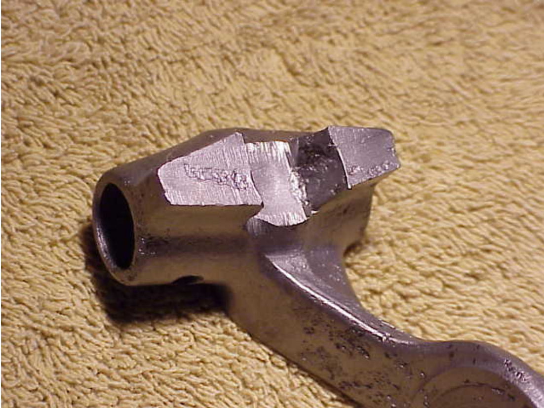
Trans tower fork worn
