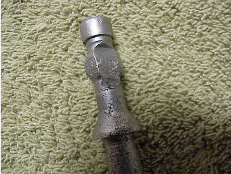
Worn ball on the end of the shifting lever
