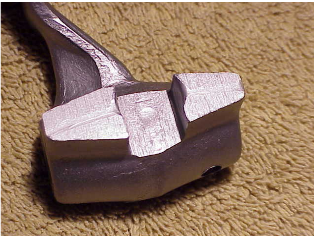
Trans tower fork worn
