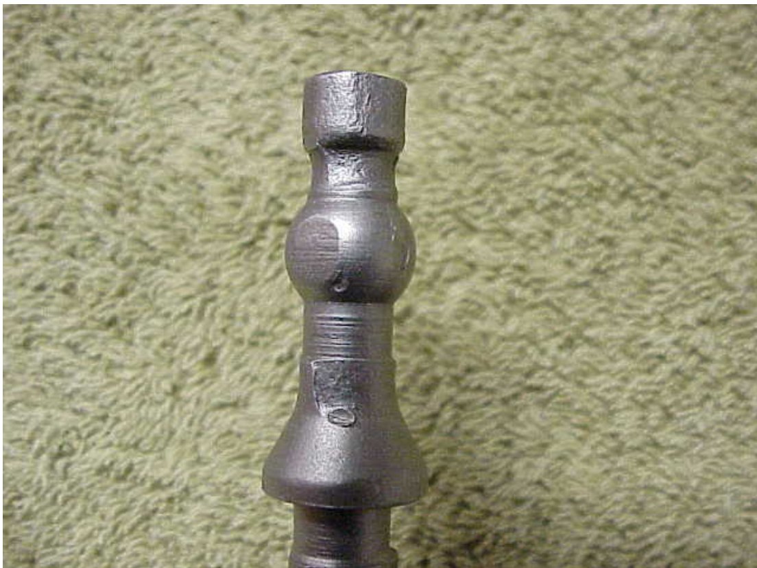
Slightly Worn .490 ball on the end of the shifter
