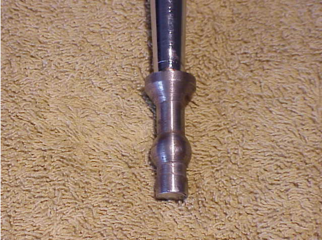
Serviceable ball shown on the end of a new reproduction shifting lever
