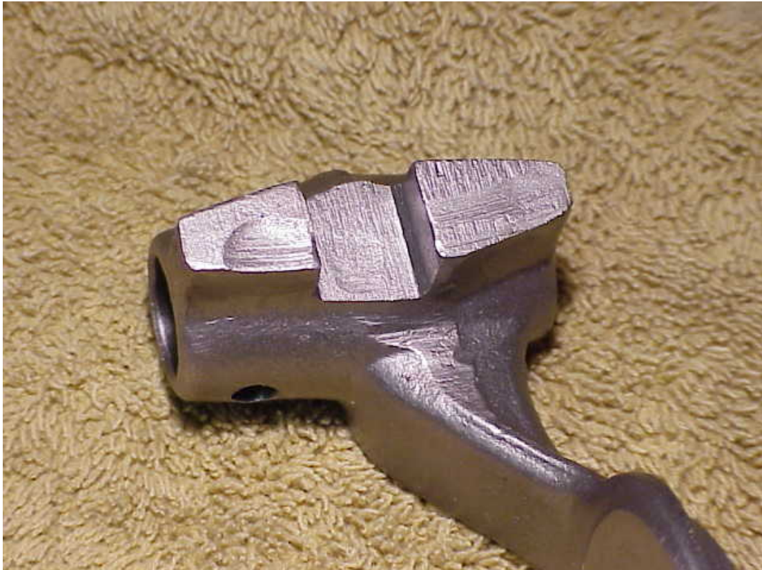
Trans tower fork worn
