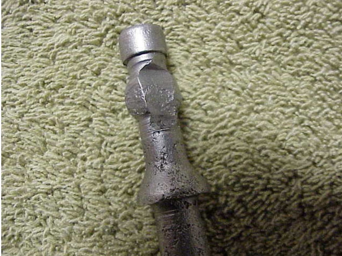
Extremely worn .490 ball on the end of the shifter
