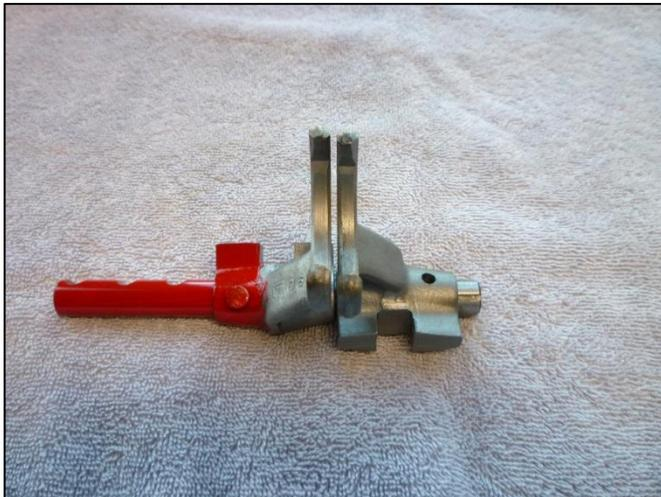
**Two known good shifting forks are assembled as seen in the photo. The one on the left is pinned to the shaft and painted red and is the reference fork. The one on the right is a fork being tested and is also a known good fork. It is slid onto the shaft in the manner shown. Note there is a nominal 1/16" space between the legs of each fork. The fork on the right being tested can be rotated and the space will remain even.**
