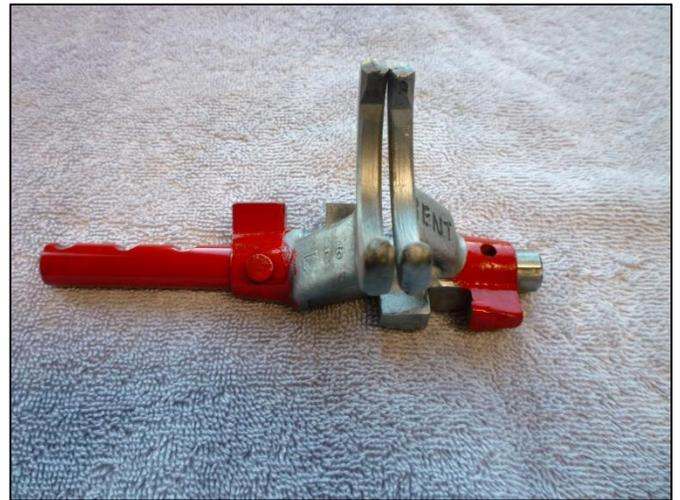
**In this photo the fork on the right being tested is known to be bent. Note that the two legs of the fork are touching at the top of the photo while there is a nominal space of 1/16" between the bottom two fork legs. The bent fork on the right can be rotated and the bent fork will strike the opposite leg.**
