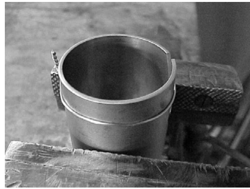
Safety wire wrapped on A4655 sleeve (Dimple on right side just above safety wire)
