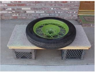
The wheel is placed on the board with the hubcap facing down into the 9" hole. To make the tire slide on the rim easy obtain a large can of baby powder. Liberally sprinkle the powder on the inside of the tire and especially around the bead. Coat the inner tube with powder as well.
