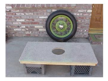
The board is made of 3\4" plywood 44" long and 21" wide. There is a boarder 1&1\2" wide nailed around the bottom edge. Two plastic "milk carton" containers fit nicely under the board and will easily support my weight along with the wheel and tire. A 9" hole is cut in the center and the surface is covered with carpeting.
