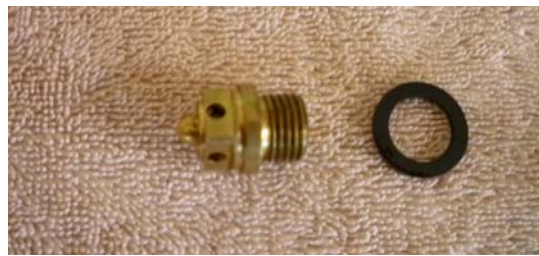
Float Valve (Viton Tip)
