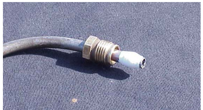
White Teflon tape is wrapped around the ferrules at each end of the fuel line
