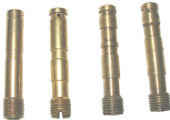
Four different style secondary wells (photo by Chris Pelikan)
