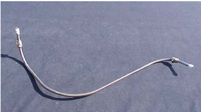
White Teflon tape is wrapped around the ferrules at each end of the fuel line
