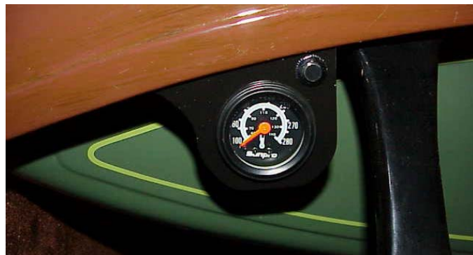
The little switch in the upper right corner of the bracket is a momentary push button switch wired to the ammeter that will give you a quick peek at the gauge while driving at night.
