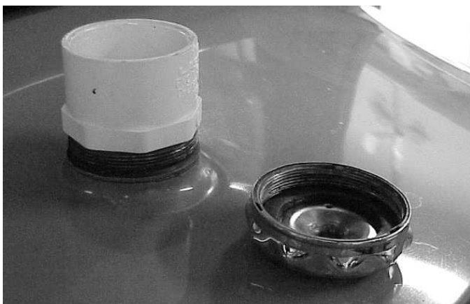
PVC pipe fitting in gas tank filler opening
