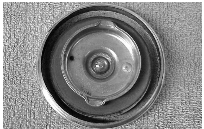
Modified gas cap with a small rivet epoxyed into place opposite from the vent hole.
