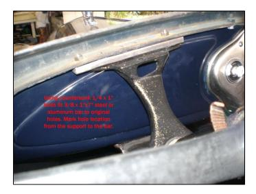
The adapter can be fabricated from either steel or aluminum. It should be one inch wide, seven inches long, and  $3\8$  inches thick. Four holes are drilled in the adapter. Use four  $1\4-20$  countersunk bolts, one inch long, along with four nuts and lock washers.
