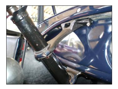
For the 1930 and early 1931 cars the later column support will bolt right up to the existing bolts in the dash rail.
