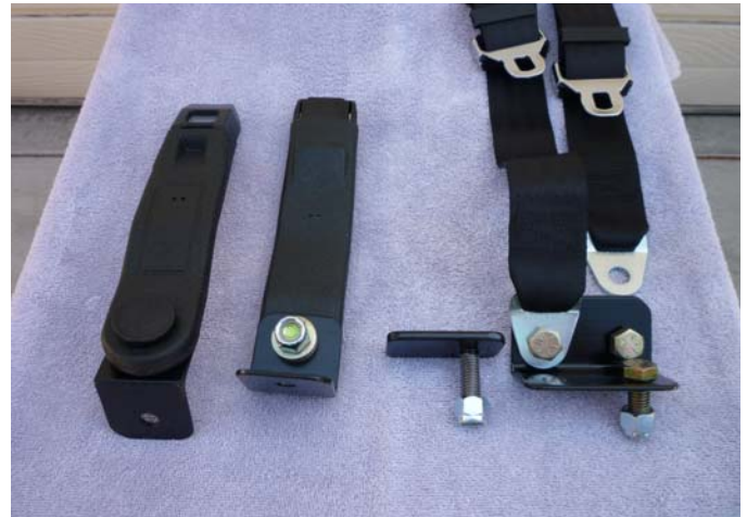
The complete seat belt installation hardware including the purchased seat belts and the fabricated L-bracket hardware.
