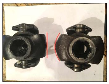
The U-joint on the left is correct; the U-joint on the right is incorrect. Note the protrusion on the sides.
