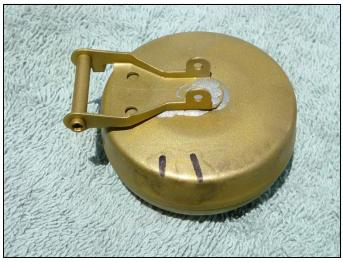
Good grief! And that's what it was. That hairline crack shown on the top of this Zenith float caused it to fill up with gas over time until it finally sank and flooded the carburetor.
