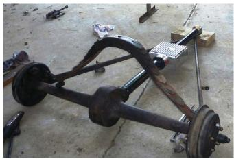
Fortunately the spring was still attached to the frame of the car when the shackle broke.
