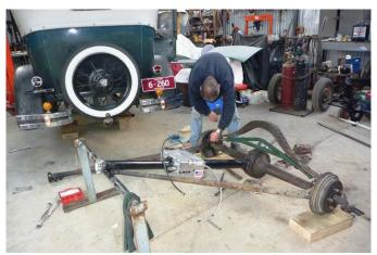
A proper spring spreader was obtained to reinstall the spring. The hazard here is the 86-year-old 3\8" rusted center bolt may be ready for the head to pop off. If it were to do so the top leafs will fly 20 feet in the air and possibly injure the fellow working over the spring. If he escaped injury he needs to run like the devil, because they will be coming back down.
