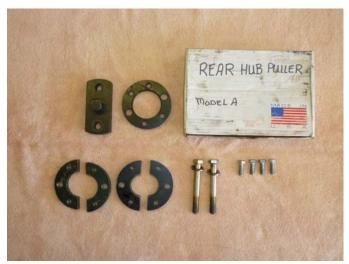
The Mitchell rear brake drum pulling tool: The two C-shaped parts (painted green on the left) are used to configure the tool to pull the shoulder and tapered design hubs. The two C-shaped parts (panted black on the right) are used to configure the tool to pull the grooved designed hubs.
