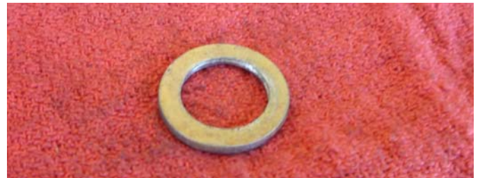
Fig.4 The shims that were used have an inside diameter of .450 and an outside diameter of .750. They fit very neatly between the emergency carrier and the grease baffle.
