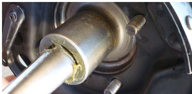
Fig.2 This is how far the bolts protrude through the backing plate and the emergency brake carrier. The grease baffle, which is very thin, has not been installed yet.
