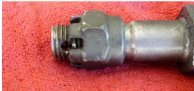
Fig.1 Shows the castle nut run all the way up on one of the mounting bolts. The hole protrudes way past the end of the castle slot in the nut. This is often how the relationship of the bolt and nut ends up after the backing plate, emergency brake carrier, and grease baffle are installed.
