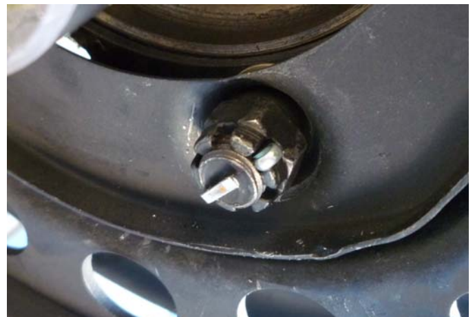
Fig.5 The final photo shows the backing plate installed using a nominal .020 of shims on each bolt between the emergency carrier and the grease baffle. The castle nut is properly aligned at the end of the mounting bolt and the cotter pin installs neatly. ©
