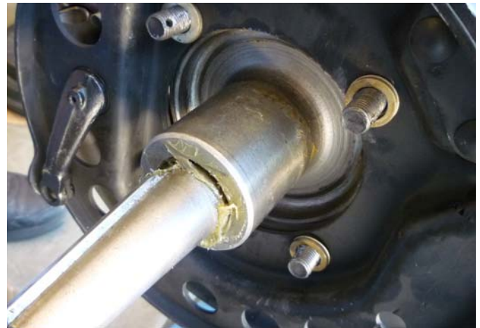
Fig.3 Special shims have been added on each of the four mounting bolts before the baffle is installed. The total thickness of the shim stack is a nominal .020" in thickness. This will space the castle nuts out further on the bolts and better align them with the cotter pin holes. It will also ensure that the nuts have not bottomed on the threads of the bolts.
