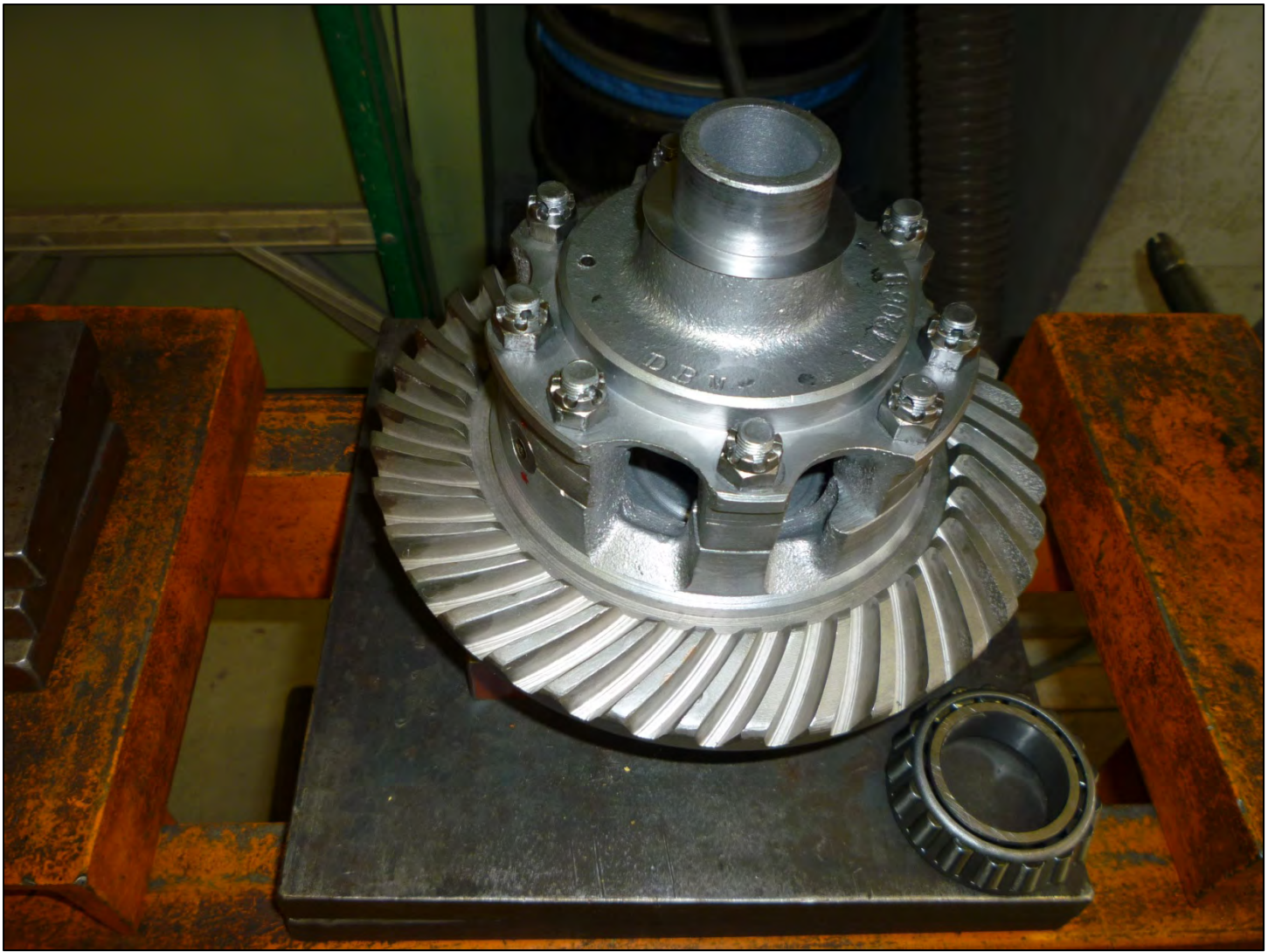
The carrier is placed back on the press and a .005 metal shim installed under the bearing.
