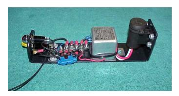
The complete assembly is shown above. The inverter is the square looking device in the center. The power outlet is to the right. The power outlet points straight down when installed under the dash rail. A single wire runs from the terminal strip to the negative 6-volt battery voltage. The power switch and the indicator lamp are to the left. The entire assembly is grounded by virtue of mounting it under the dash rail.
