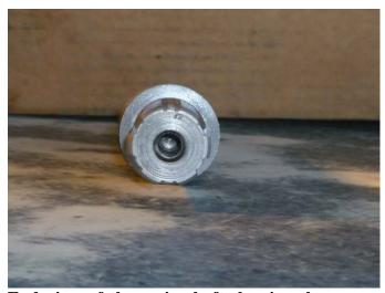
End view of the main shaft showing the spaces under the bearing stop.
