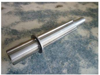
Note the spaces under the bearing stop on the main shaft. There is a space under each flute for the two sliding gears.
