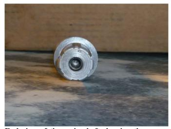
End view of the main shaft showing the spaces under the bearing stop.
