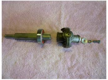
The U-joint is attached to the end of the main shaft and acts as the rear bearing stop. The notched washer fits around the fluted end of the main shaft and is what prevents oil from escaping from the transmission.
