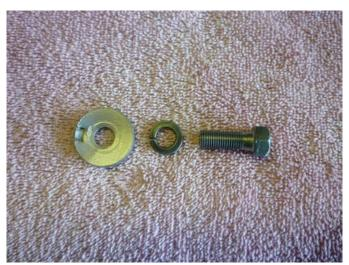
The special flat washer with the notch is used in conjunction with the bolt and lock washer that attaches the U-joint to the rear of the main shaft.
