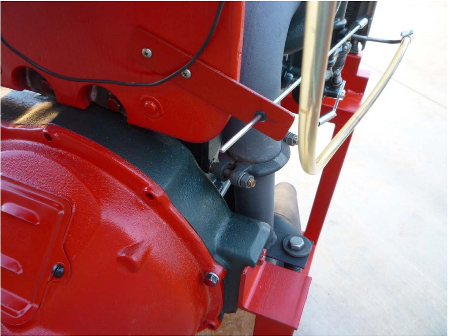
The throttle control rod can be seen at right; The O-ring provides enough restriction to hold the rpm level in place where set.
