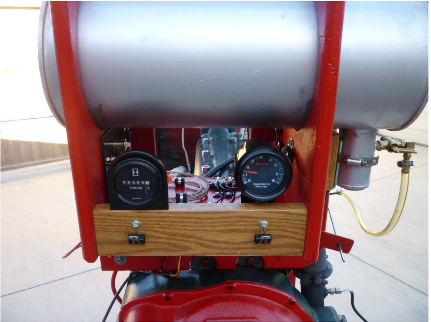
The fuel tank is mounted to the top of the control board. A tool tray is located above. The running time meter and tachometer are located below the fuel tank. Running time meter on the left, tachometer on the right.
