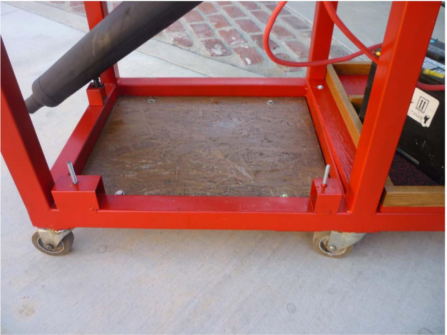
Two mounting studs are provided to store the radiator on when there is no engine in the test stand. The platform behind is used to store other components when there is no engine in the test stand.
