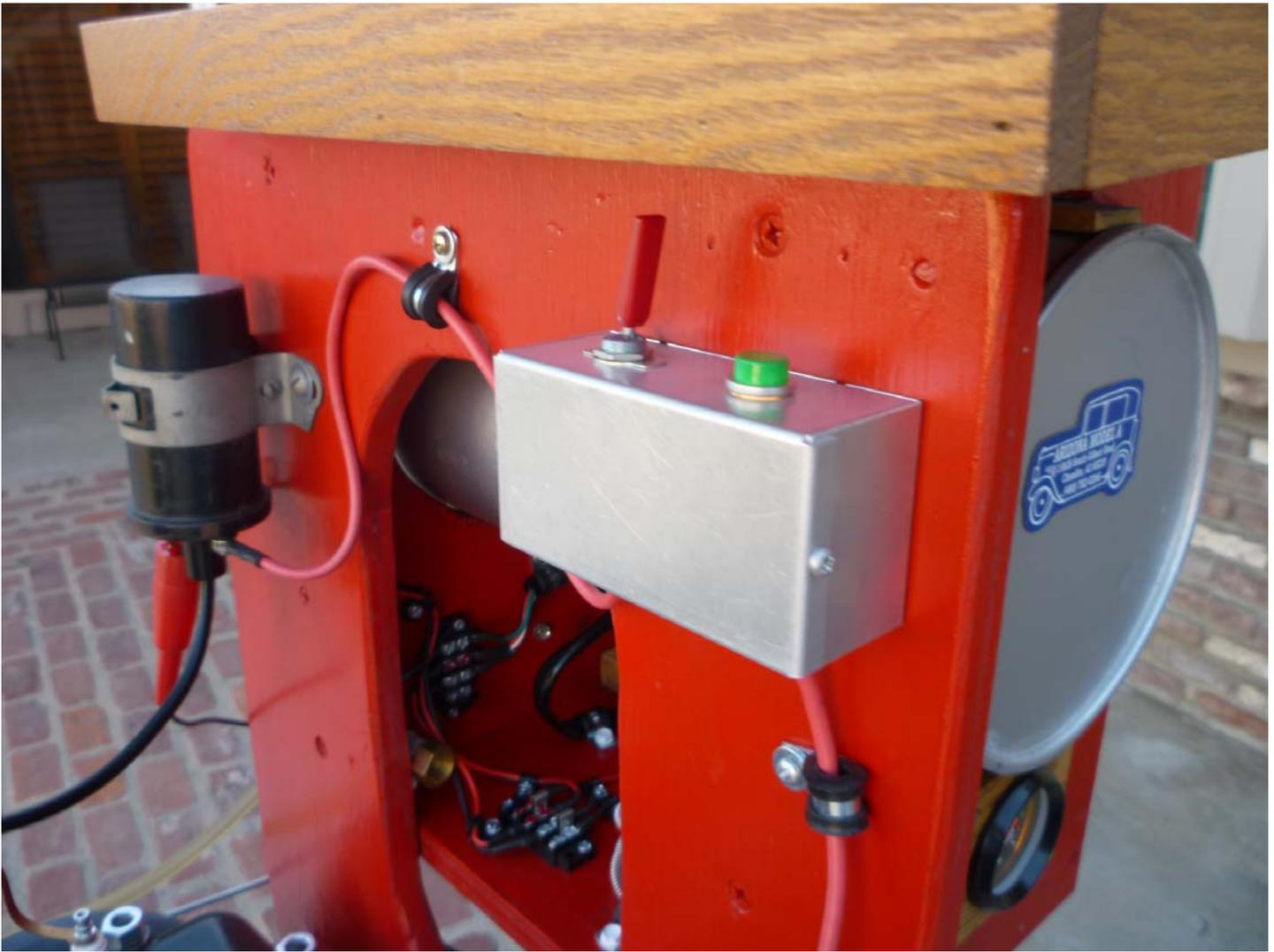
The ignition control panel is shown at right; the 12-volt coil is mounted at left. The water temperature gauge can be seen below the fuel tank at right on the right side of the mounting board. The red handled switch is the ignition switch.
