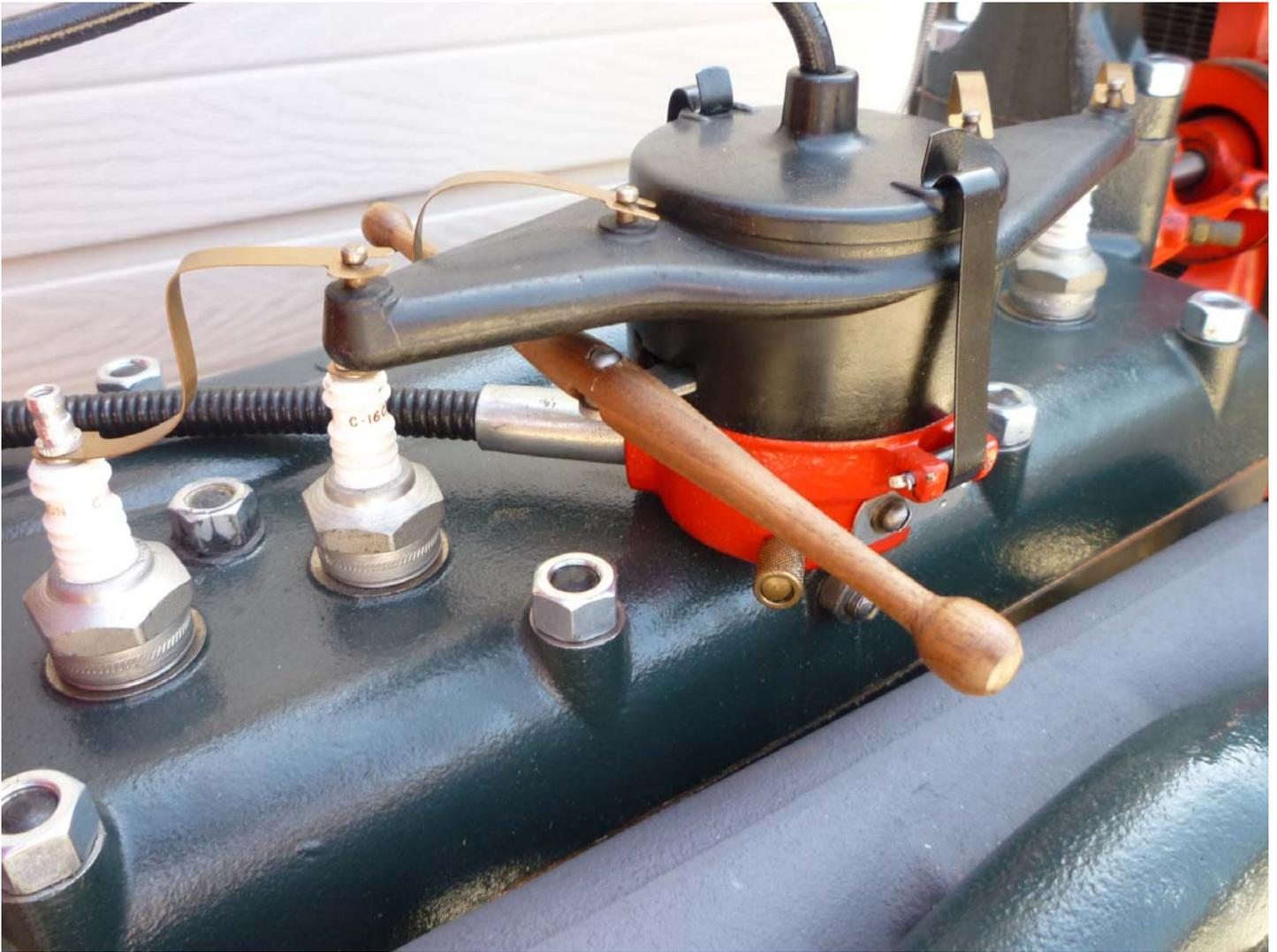
The timing advance rod is exquisitely made of the finest hardwood by Bryan Thompson such that it can be adjusted from either side of the engine without encountering a spark plug or hot exhaust manifold.
