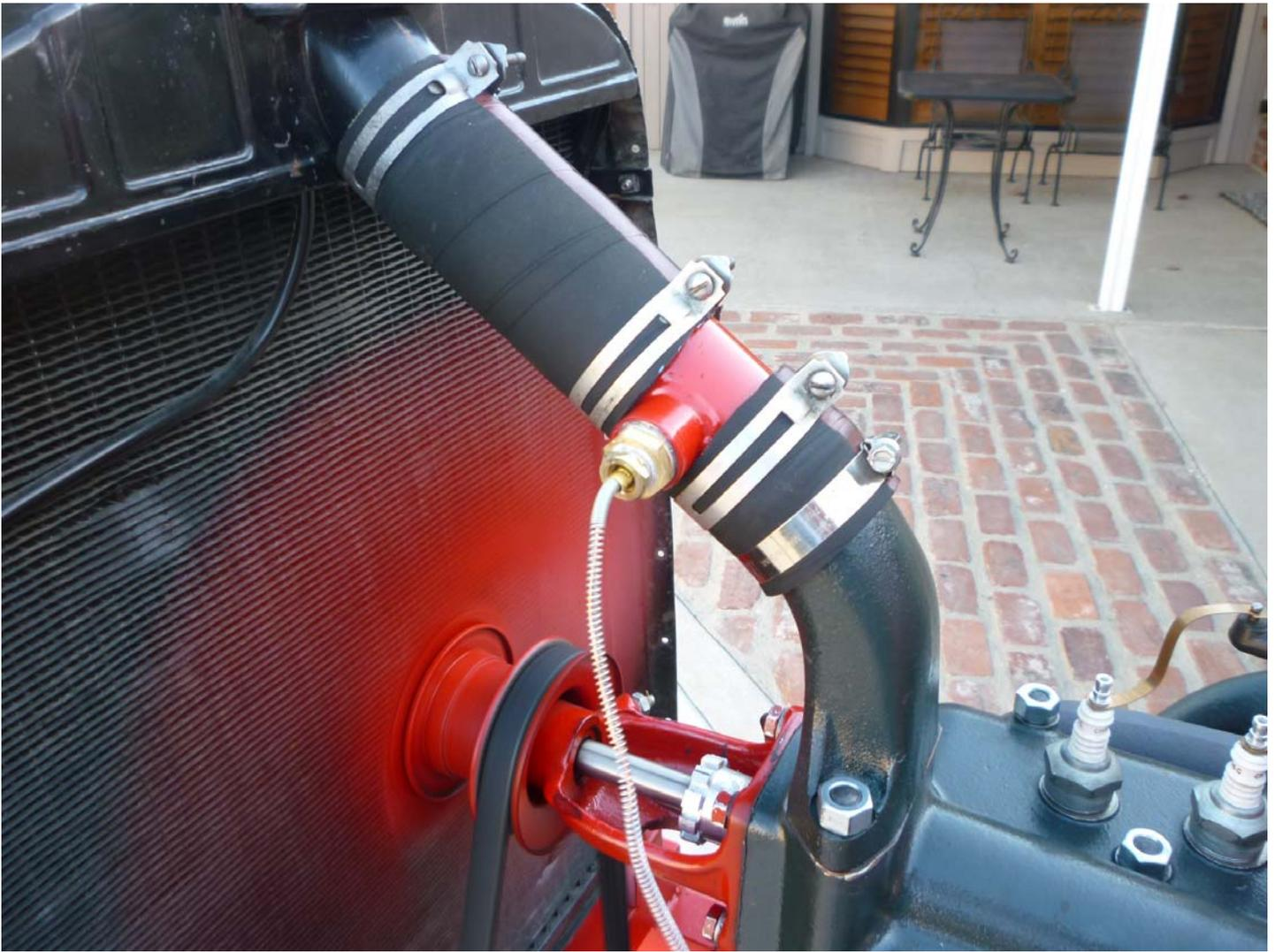
A boss is shown inserted into the water outlet hose to accommodate a water temperature probe that is connected to a temperature gauge.
