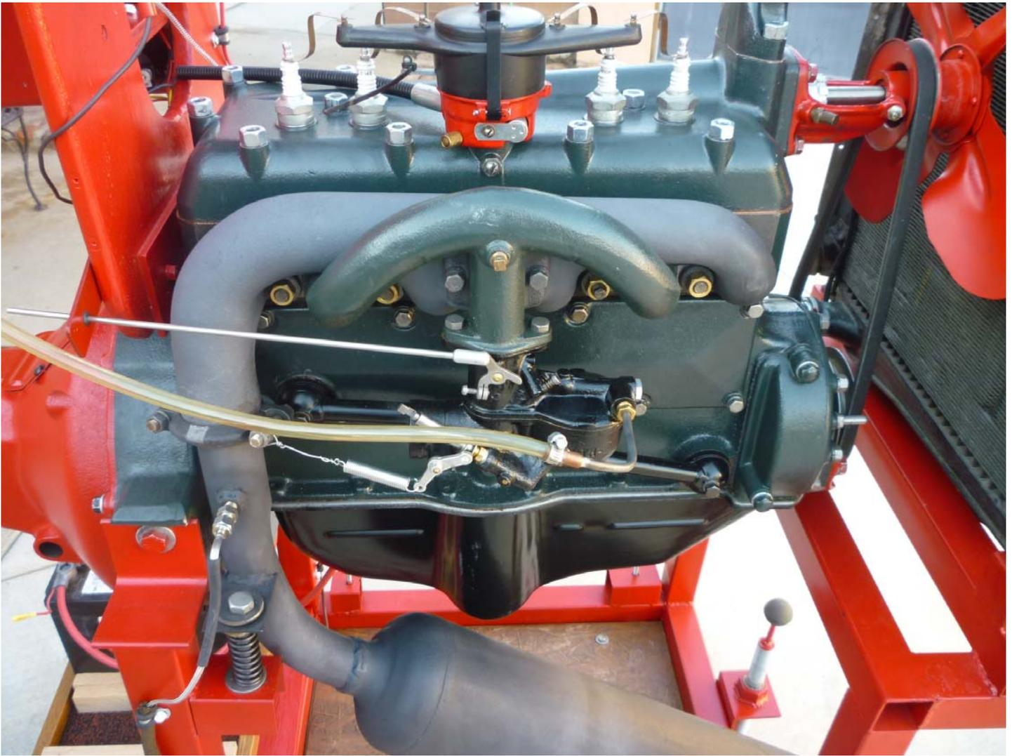
The spring load mount for the top side of the muffler can be seen at left. The muffler remains in place whenever there is no engine in the test stand. A temperature probe for an EGT meter is installed two inches down from the muffler clamp. The probe remains in place when the engine is removed from the test stand.
