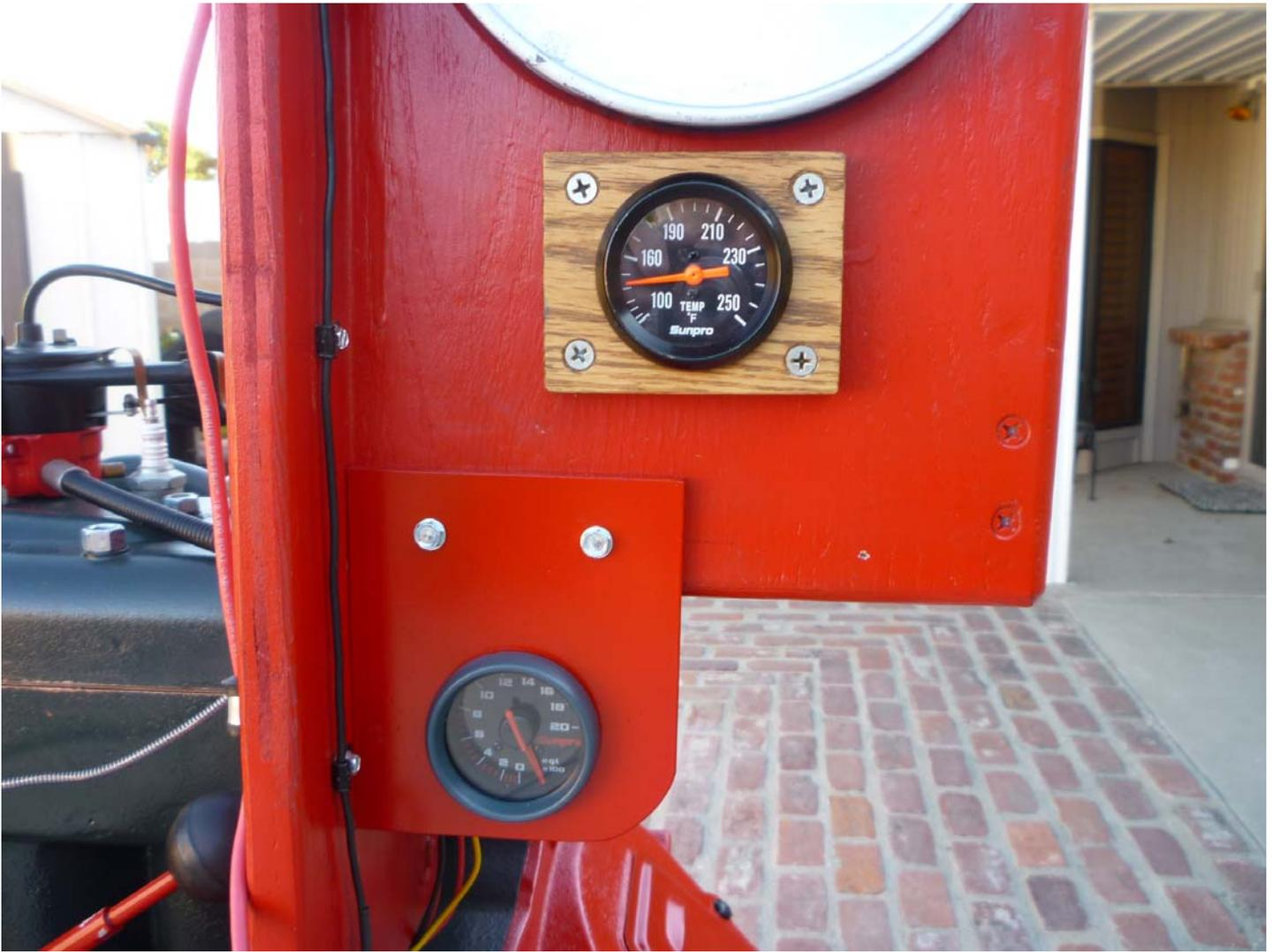
The water temperature gauge is mounted to the left side of the control board just below the fuel tank. The gauge contains a backlight connected to 12-volt power for nighttime operation.
