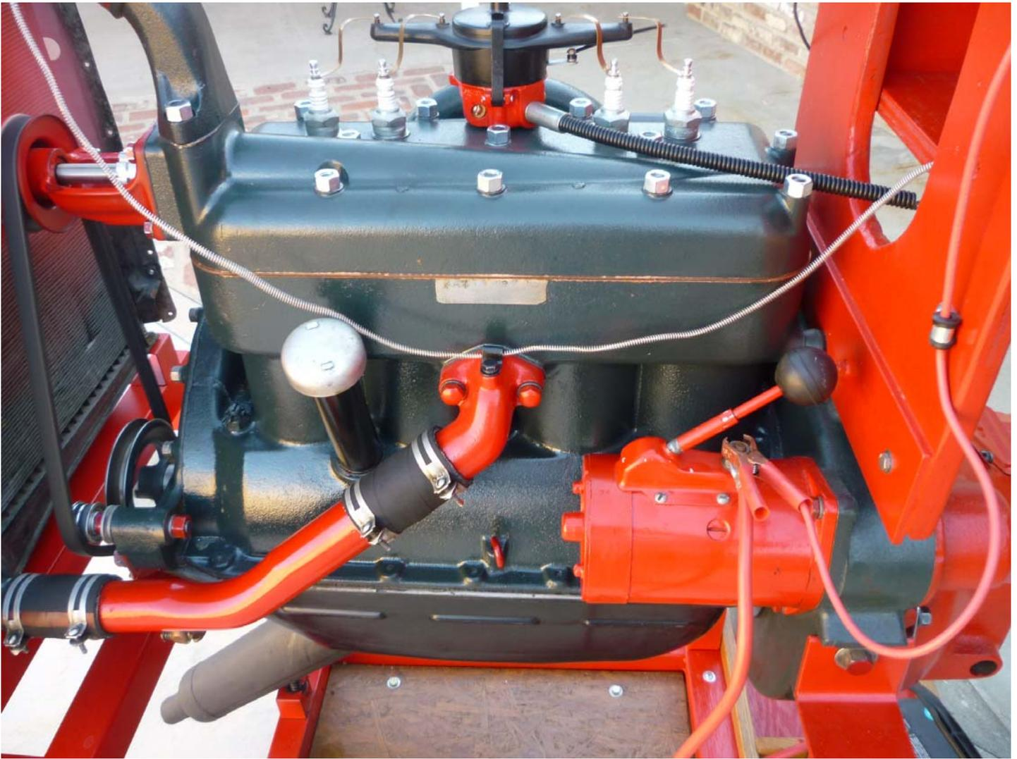
The starter is hand operated by pushing on the Model A gear shift knob attached to a short rod.
