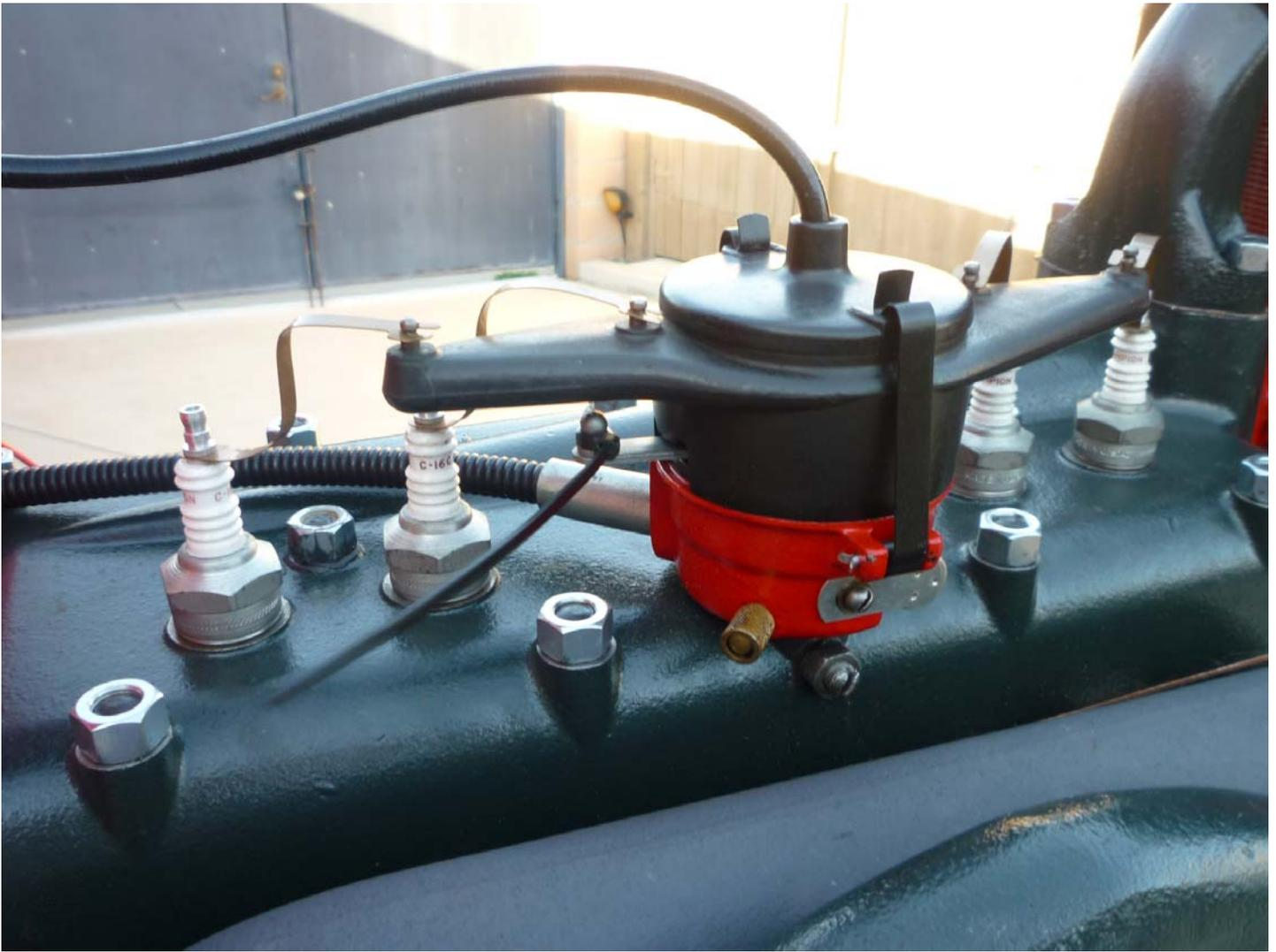
The distributor has a tie wrap attached to the spark advance lever for convenience of setting the advance. When timing a test engine the distributor upper section has to be temporarily mounted and the spark advance lever pulled toward the manifolds until it is up against the stop. This is the fully retarded position and duplicates the position it would be in if it were connected to the advance lever in a Model A.
