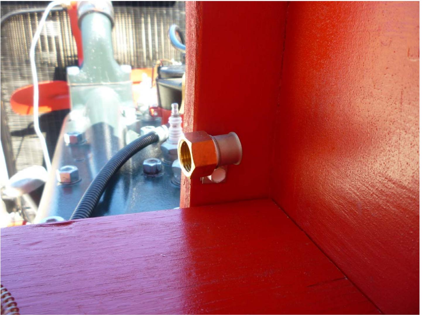
A dummy temperature gauge fitting is added to store the temperature gauge probe whenever there is no engine in the test stand.
