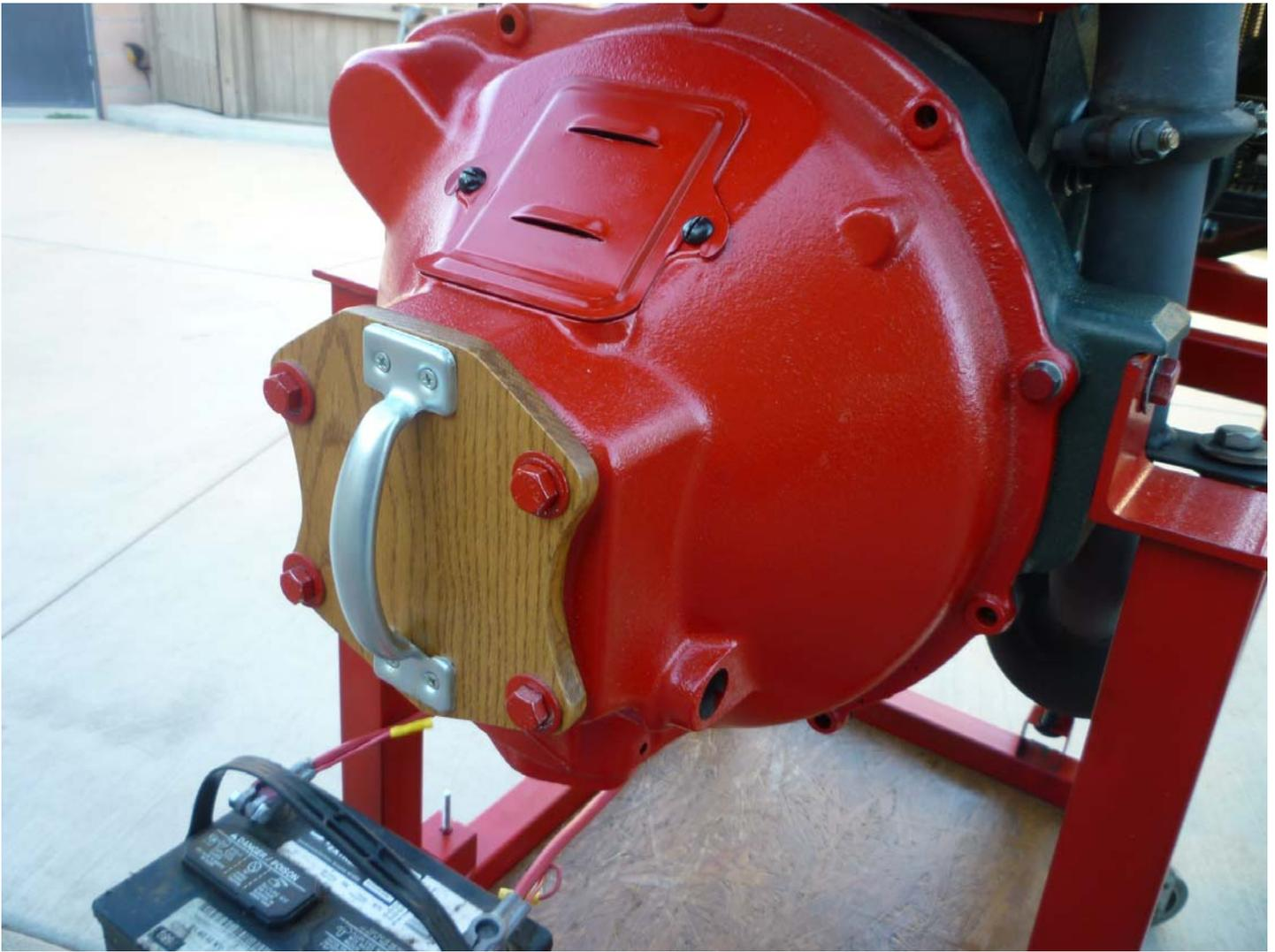
A dummy bell housing is installed as a safety feature to enclose the flywheel. The handle is used to facilitate moving the test stand around.
