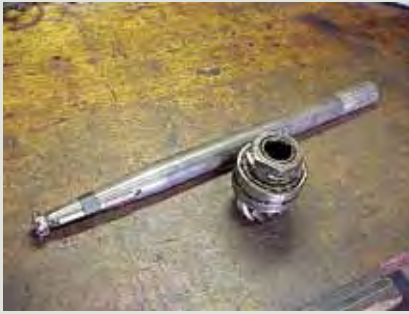
#17. The Mitchell stub shaft is inserted into the pinion in place of the drive shaft. Torque the 15\16" hex nut to a nominal 100 foot-pounds.
