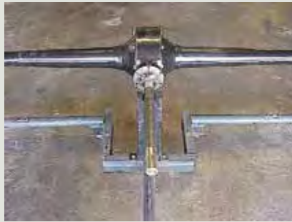
#20. Rear axle assembly with Mitchell stub shaft installed is ready for the overdrive assembly to be installed. Install the spline coupler on the end of the stub shaft splines before installing the overdrive unit.
