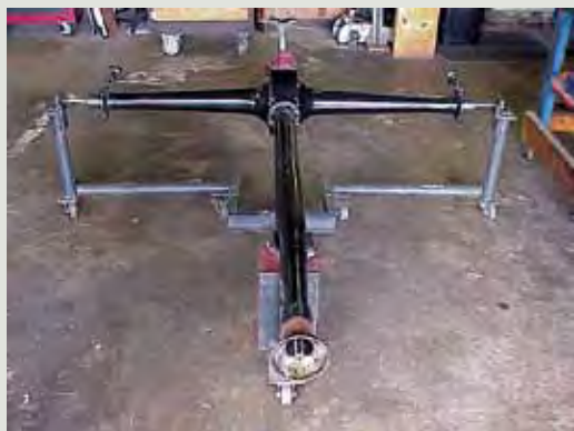
#1. The rear axle assembly is removed from the car and readied for the Mitchell install. It is not necessary to remove rear wheels, brake drums, backing plates, and rear radius rods.
