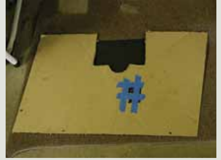
#22. A slot will need to be cut in the floorboard to accommodate the Mitchell shifting lever. Make a cardboard template to accurately locate the positioning of the slot.
