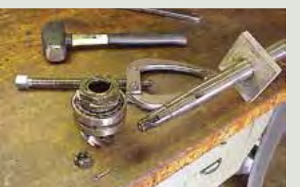
#16. The pinion assembly has been removed from the drive shaft with the existing pre-load still intact.
