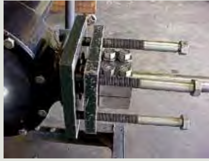
#6. Close up view of attached drive shaft puller tool.
