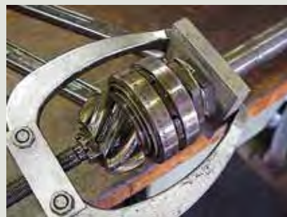
#15. A flywheel puller and a backing device are used to remove the pinion assembly from the drive shaft. Tighten the puller sufficiently tight and tap the end of the puller with a hammer. Continue tightening and tapping until the pinion breaks loose from the taper on the drive shaft.
