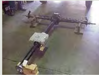
#21. The Mitchell overdrive installation is complete and the rear axle assembly is ready to be installed back in the car.
