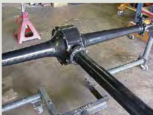
#2. Close up view. The torque tube is to be removed by removing the safety wire and the six mounting bolts. Remove the speedometer drive assembly and the snap ring in front of the speedometer drive gear before pulling the torque tube off. The torque tube, drive shaft, and the speedometer drive gear assembly will be discarded. Speedometer operation will be obtained at the output gear of the overdrive. An extension speedometer cable is supplied with the Mitchell overdrive that will connect to the existing speedometer cable.
