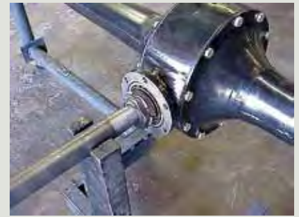
#19. Close up view of installed pinion assembly and Mitchell stub shaft.
