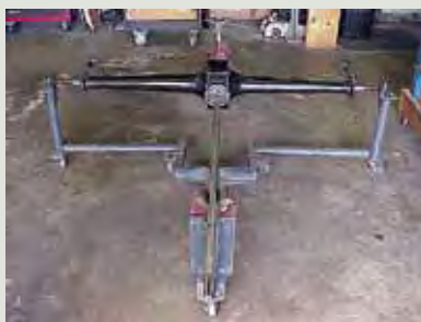
#3. The torque tube has been removed exposing the drive shaft.
