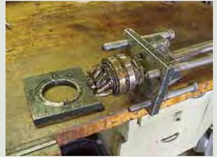
#10. The removed drive shaft with pinion assembly is clamped in a vice and the puller tool removed.
