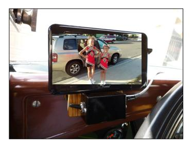
The screen is positioned to the left side of the dash rail with a U-shaped oak fixture that straddles the rail. The switch on the left side of the chassis box powers both the screen and the camera. The cable connector on the right side of the chassis box is easily disconnected.
