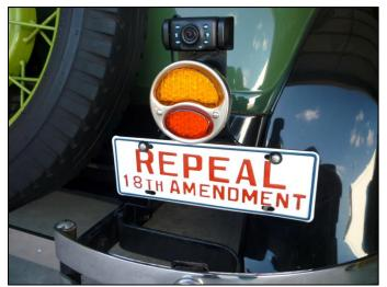
The Yada camera is mounted above the right tail light, is vertically adjustable and has night vision capability.
