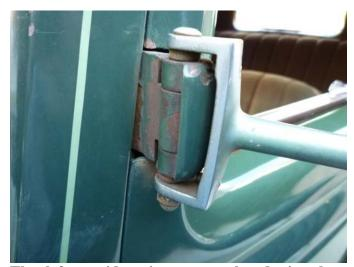
The left outside mirror was already in place when I obtained the car years ago. I don't know what the diameter of the hinge pin is as I am reluctant to want to take it apart to find out. The mirror bracket has a hinge space of two inches. Two shims, one at bottom and one at top had been installed to obtain a proper fit.
