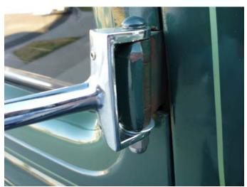
The right outside mirror bracket has a hinge space of an inch and three quarters. A .010 shim (washer) was inserted to obtain a proper fit. The new hinge pin is .300 in diameter with the bottom end threaded for the  $1\4-20$  acorn nut supplied with the mirror.
