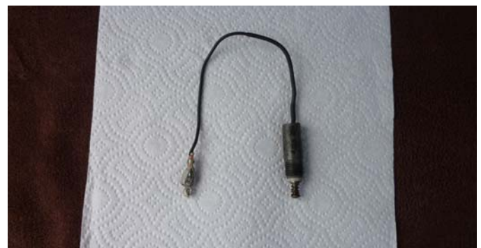
Ignition bypass cable
