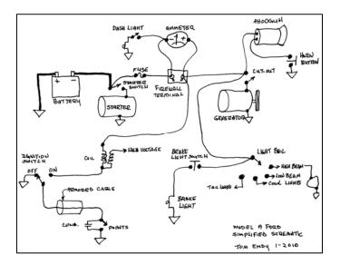
Looking at the diagram above, start at the starter switch where the battery cable attaches. Next check both sides of the fuse. Move to both sides of the terminal box on the firewall. All of these points should light the trouble light. Next check both sides of the primary of the coil. With the ignition key off both sides should light the trouble light. Put a business card between the points and turn the key on. Put the trouble light probe on the arm of the points, the light should light.
