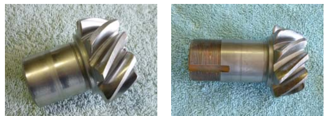
Comparison of early and late pinion gears. Early on the left, late on the right.
