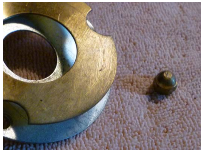
The modern lower plate. Note the witness marks on the plate and on the end of the acorn nut. This arrangement was cleaned up after it actually failed.
