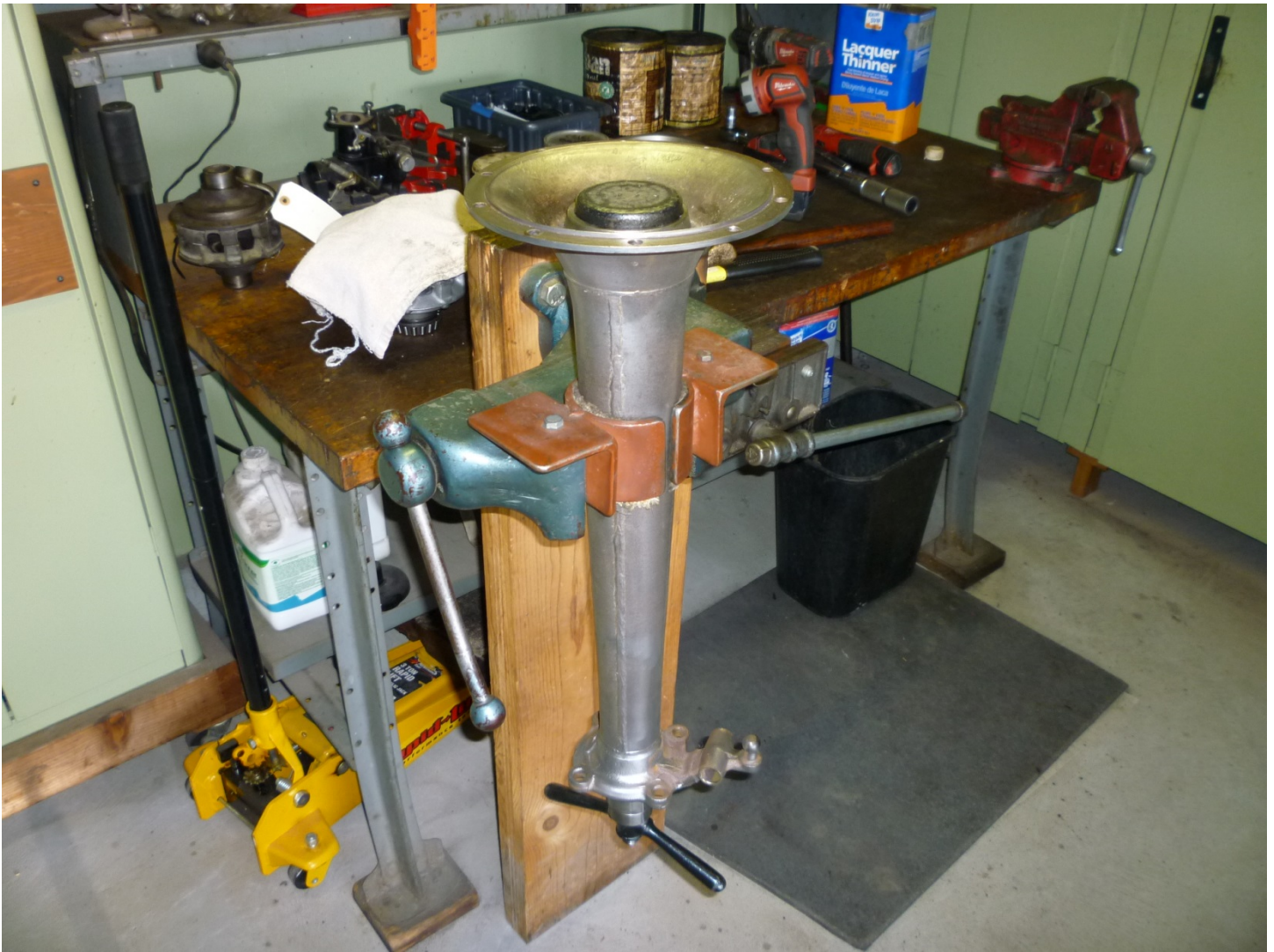
An axle housing bearing race is installed using a vintage K. R. Wilson press-in tool
