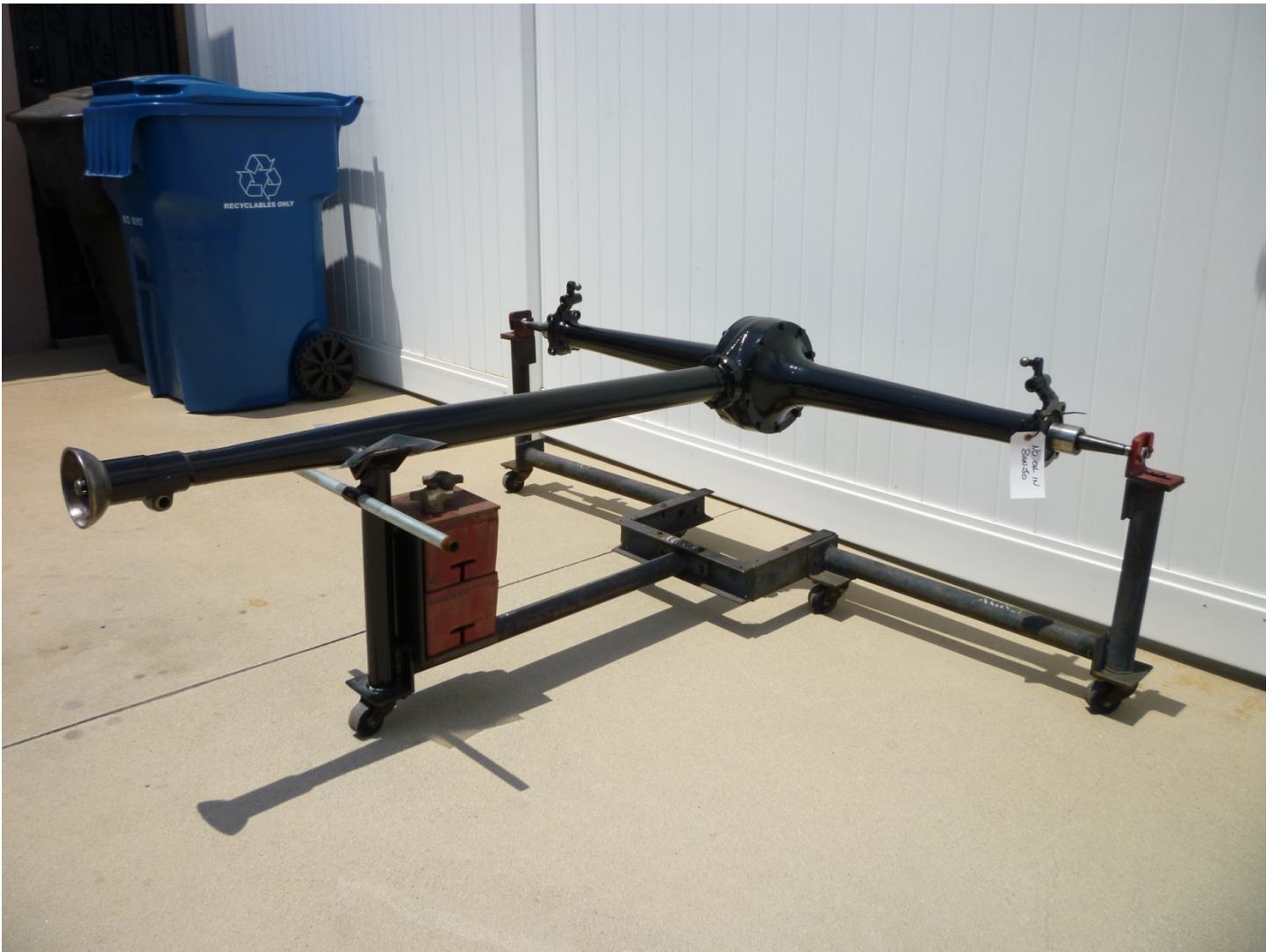
The rear axle assembly is painted and ready for return to the customer. Note the tag attached: “no oil in banjo”. Best to leave it in place until the assembly has been oil serviced.
