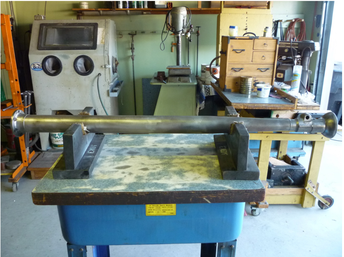
The torque tube has been cleaned up and wire wheeled to remove surface rust. The roller bearing race sleeve and the old grease seal have been removed.
