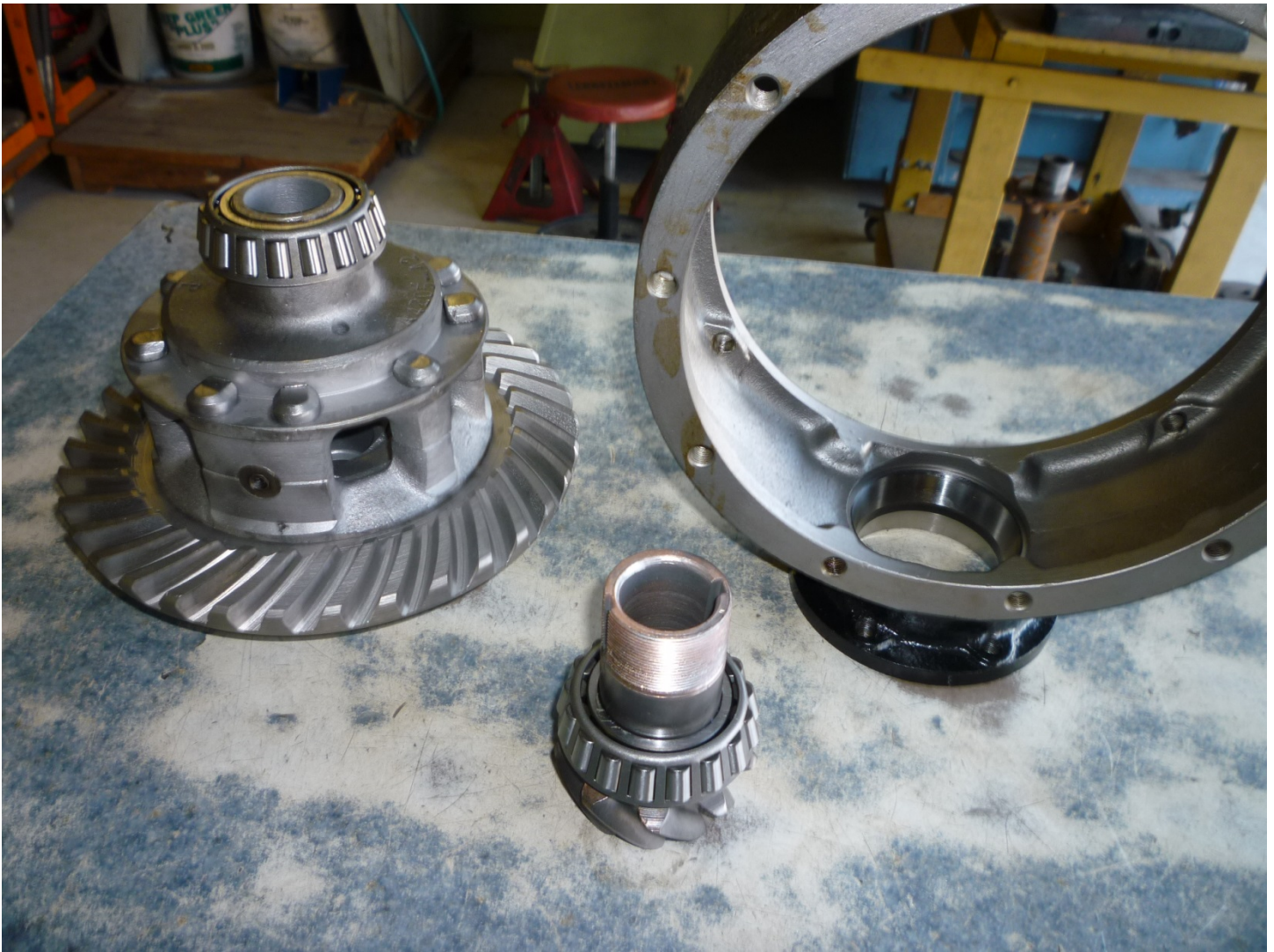
The carrier assembly with the ring gear installed. Both bearings are installed and the pre-load tool is inside the carrier. The pinion gear has a new rear bearing installed. A replacement banjo has a new double race installed.
