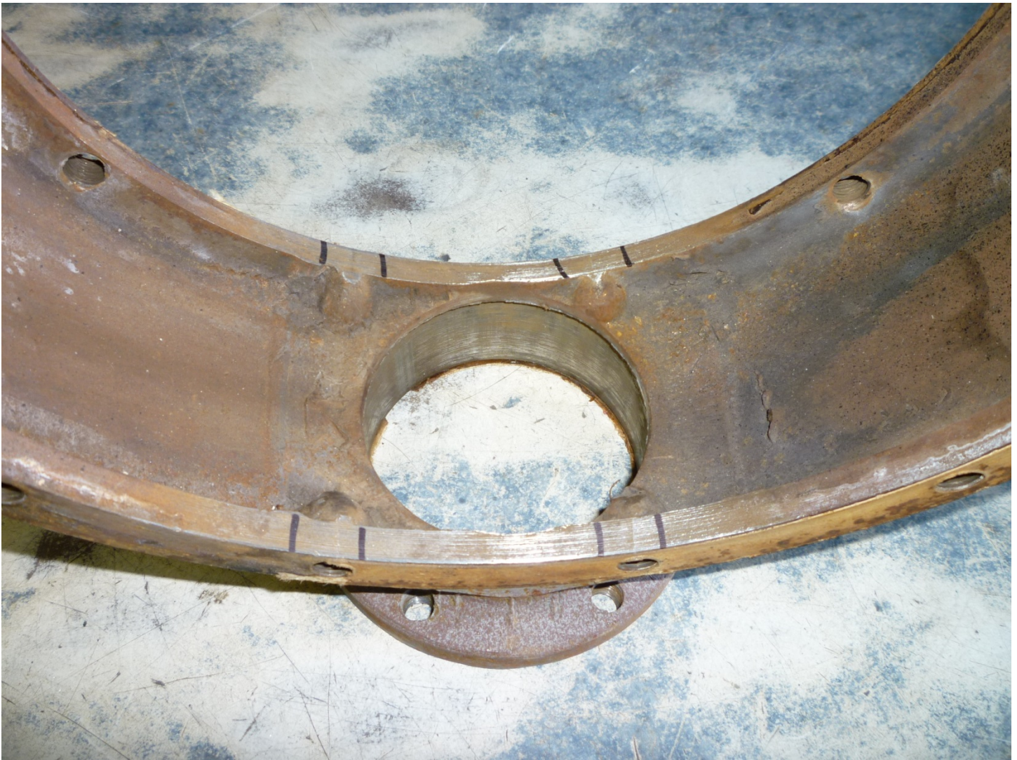
Note the four cracks across the rails at each of the four bolt holes closest to the torque tube flange. The banjo has been replaced with a 1928-1930 banjo that has support gussets
