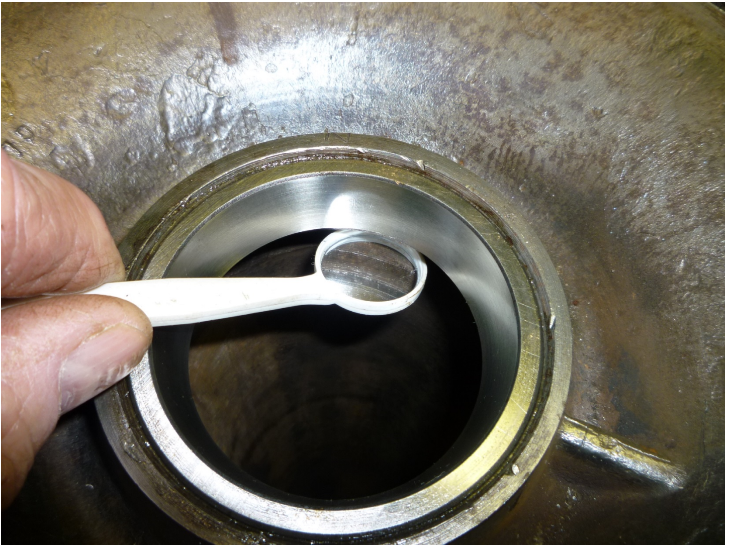
A dental mirror is used to make sure the bearing race is fully seated against the stop in the axle housing all the way around.
