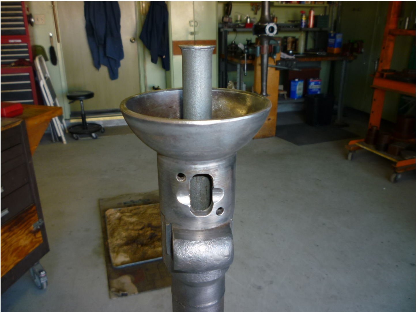
A new grease seal is driven into place with an insertion tool. The seal must be installed first before the bearing race sleeve is installed.
