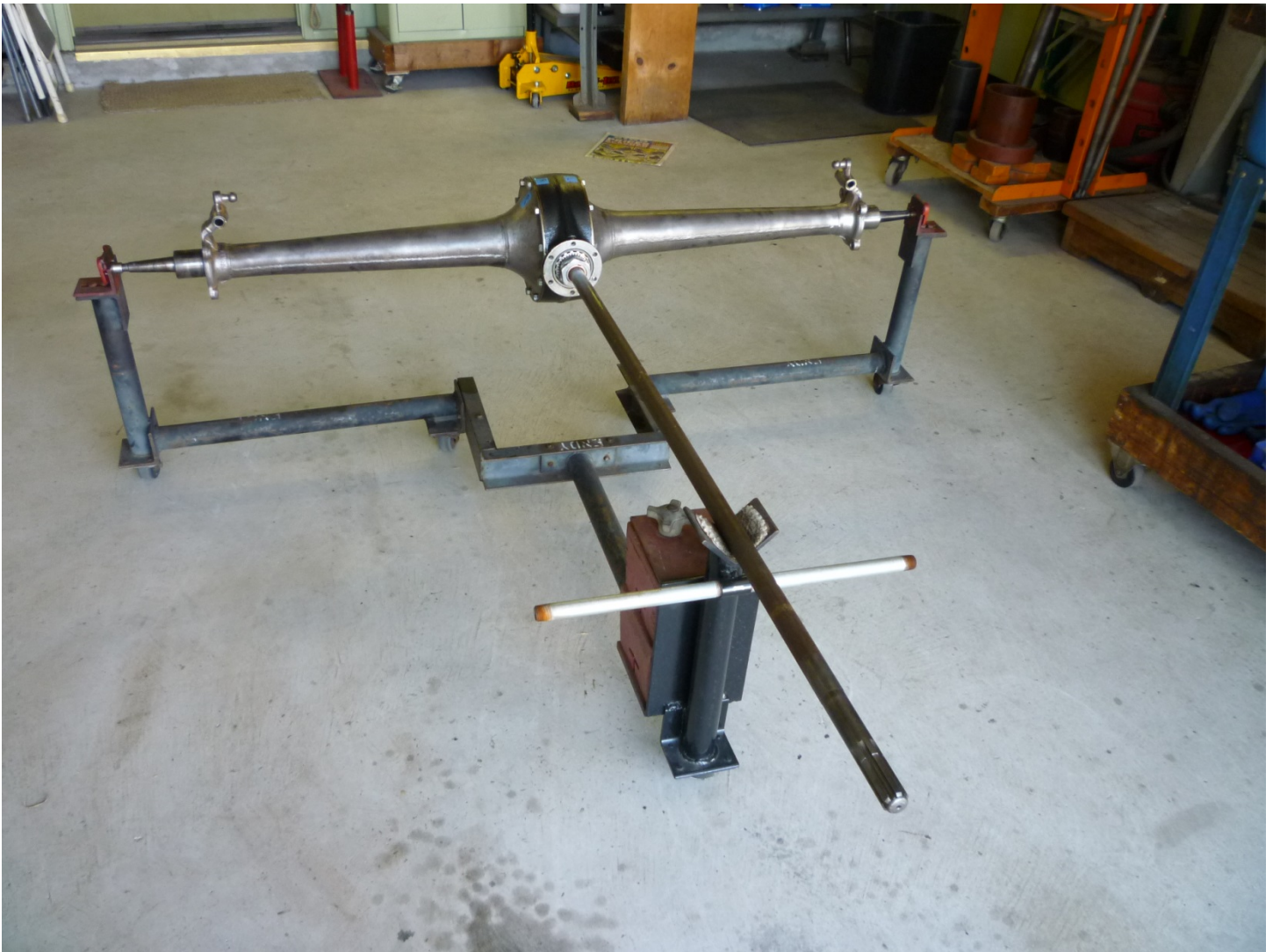
The rear axle assembly has been removed from the vertical jig and placed in the roll around cradle and is ready to have the torque tube installed.
