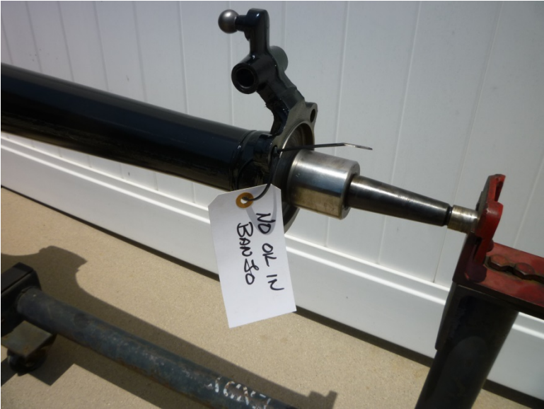
The rear axle assembly is painted and ready for return to the customer. Note the tag attached: “no oil in banjo”. Best to leave it in place until the assembly has been oil serviced.
