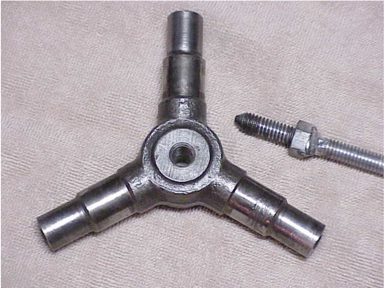
Photo P-37. Carrier bearing pre-load measuring tool: The spider gear yoke has been modified with a threaded hole that will accept the end of the threaded shaft.
