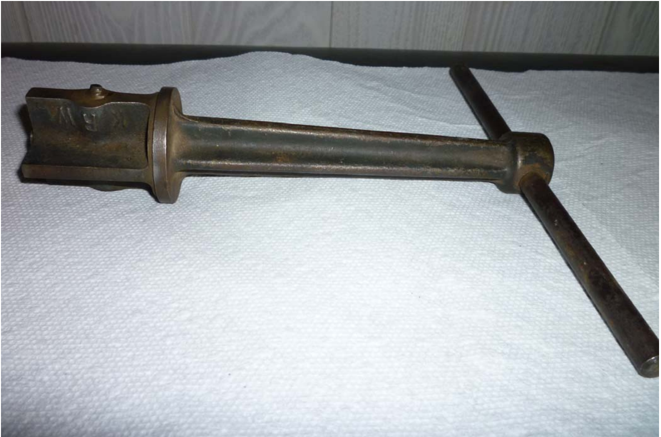
Photo P-49. The K. R. Wilson tool is used to remove and install the bearing race sleeve in the torque tube: This is an alternate option if the tool is available.
