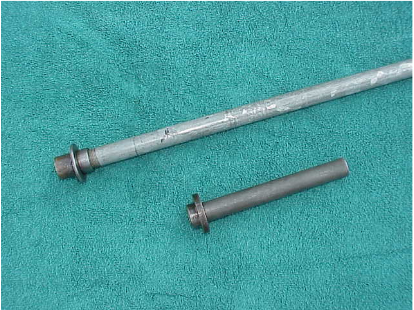
Photo P-24. Grease seal installation tools: The long tool is used to install the seals in the both axle housings. The short tool is used to install the seal in the front of the torque tube. Both tools are made from a length of 1\2'' water pipe with the seal tool threaded onto the end. A seal installation tool can be purchased from most any Model A supplier.
