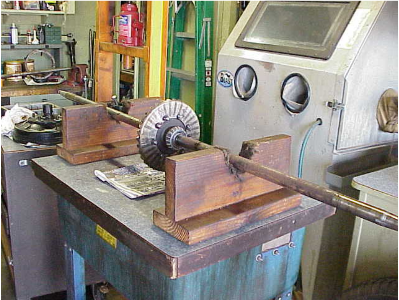
Photo P-12. Carrier disassembly: Before beginning the process, center punch both carrier halves so they can be re-assembled as before. The safety wire is removed and the nine carrier bolts are removed. When the two carrier halves are separated the spider gear assembly will drop out and the two axles can be removed. Care should be taken to not damage the threads on the nine carrier bolts. Do not hammer aggressively on the threaded ends of the bolts.
