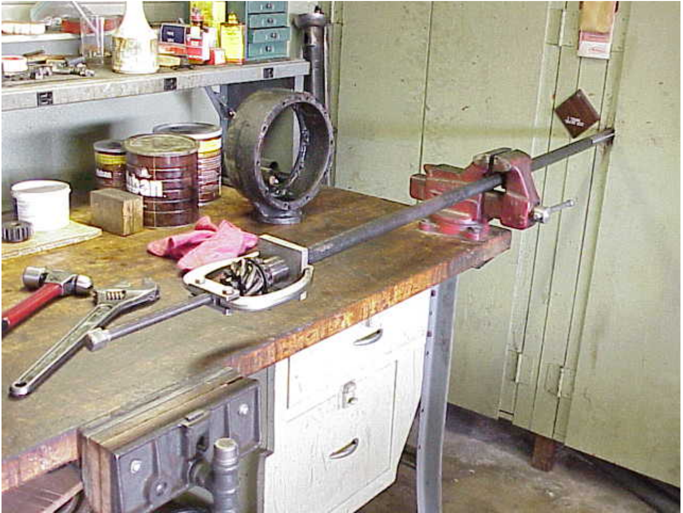
Photo P-6. Pinion gear removal: Do not remove the nut when attempting to remove the gear as it may come off and fly across the room. Once the gear breaks loose from the taper on the shaft the puller will drop free. Remove the nut then.
