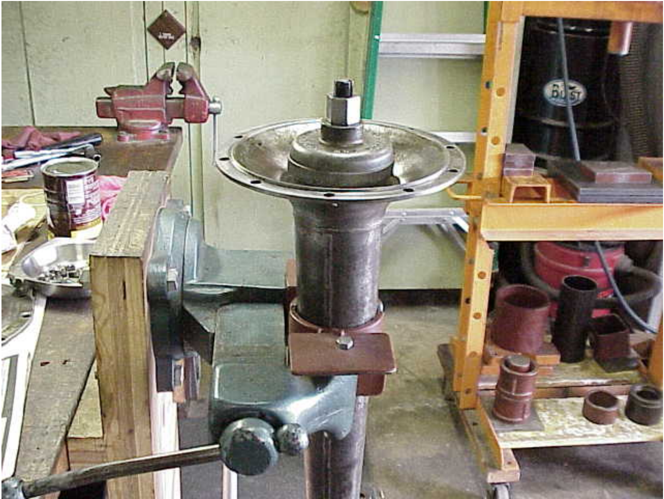
Photo P-11. Removal of axle housing bearing race: The axle housing is supported in the vertical jig for the removal process.
