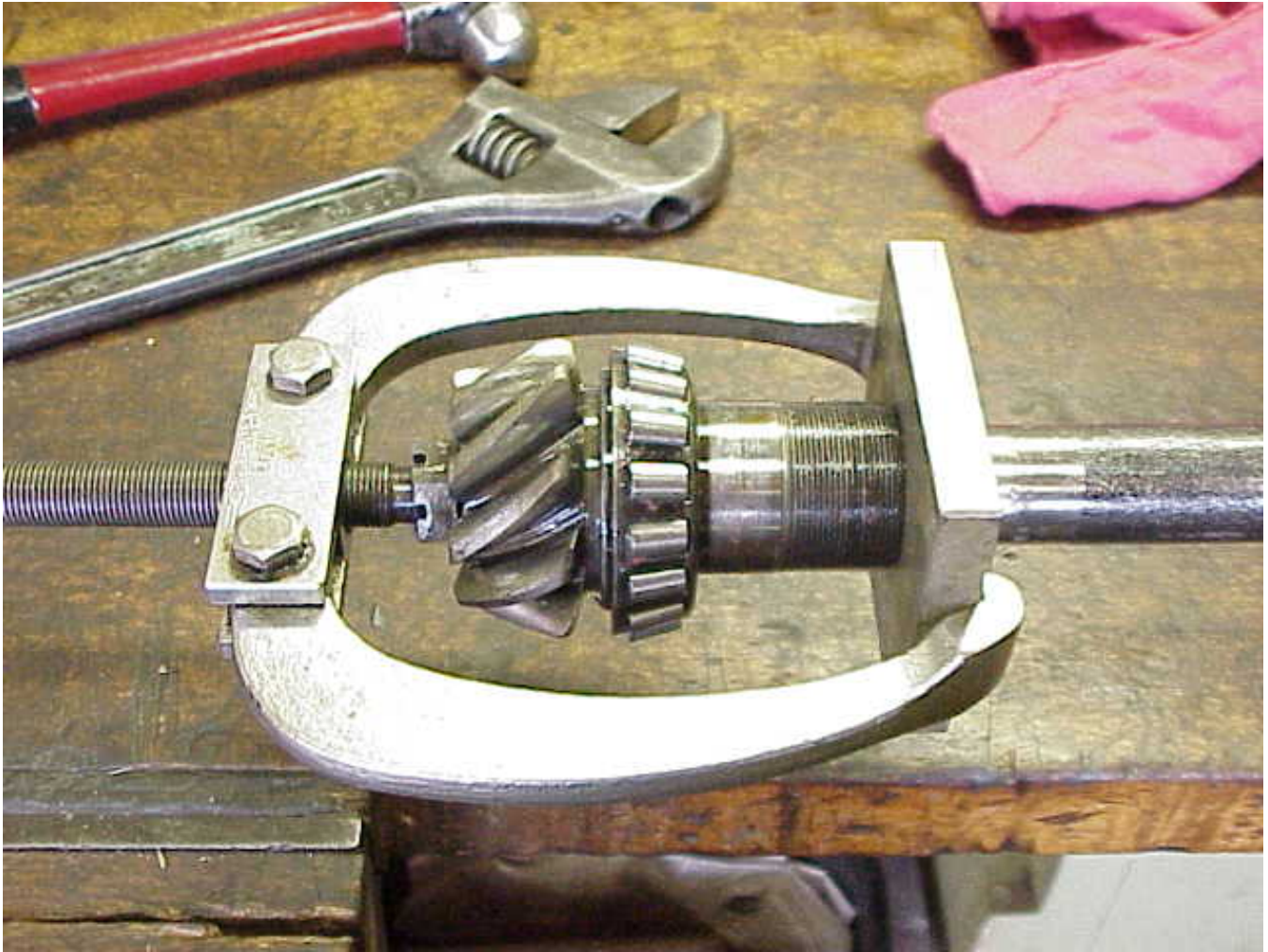
Photo P-7 Pinion gear removal: Photo 5. Pinion gear removal: Tension is applied to the puller tool; the end is then tapped smartly with the hammer. Repeat tightening and tapping until the gear comes off the shaft.
