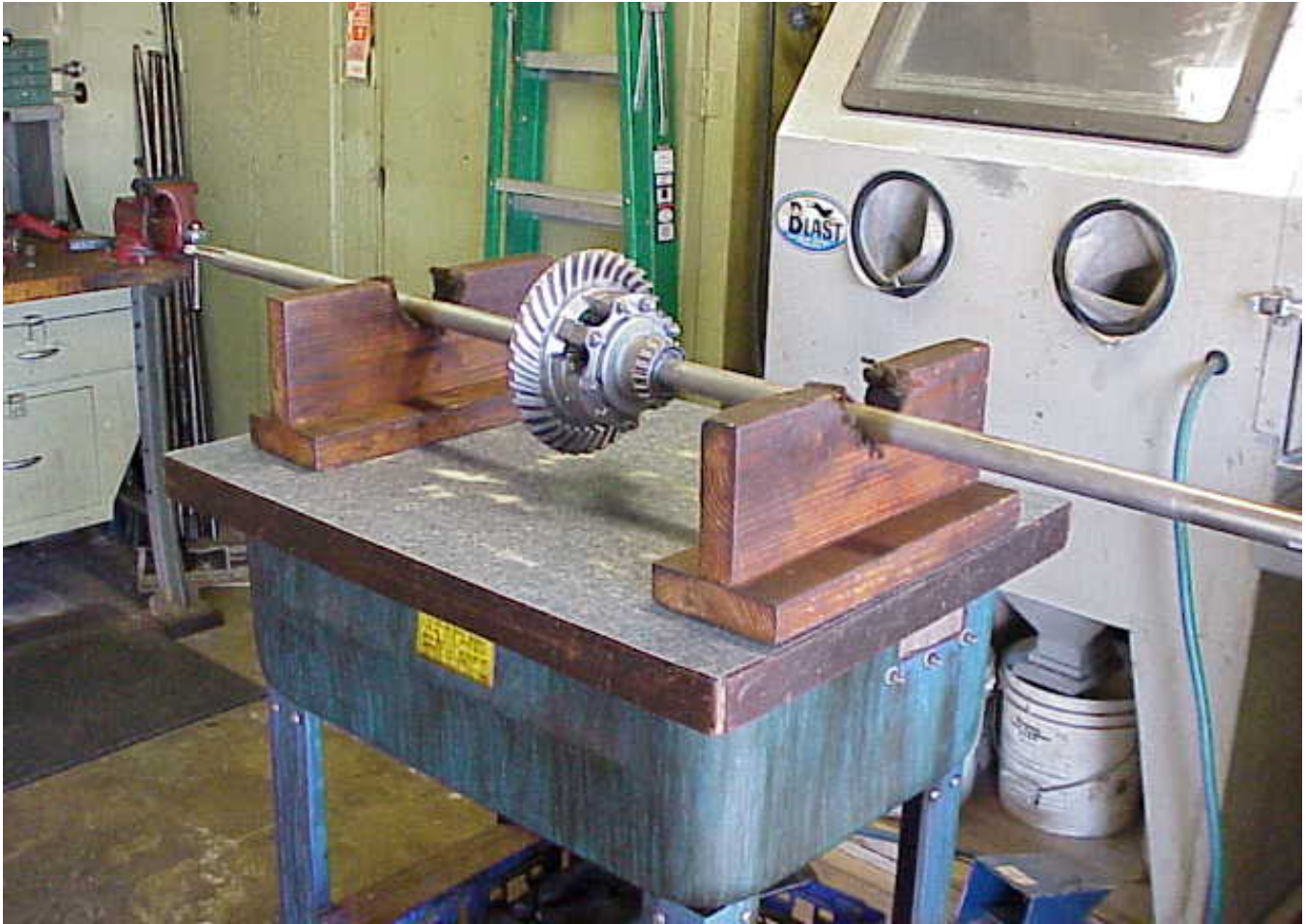
Photo P-45. Final assembly of carrier: The axle shafts and spider gears are installed: The 9 bolts are torqued to 35 ft. lbs. and safety wired. Rotate both axles by hand in opposite directions to ensure there is no binding. Note: Some reproduction axles will bind inside the carrier because they are made incorrectly.
