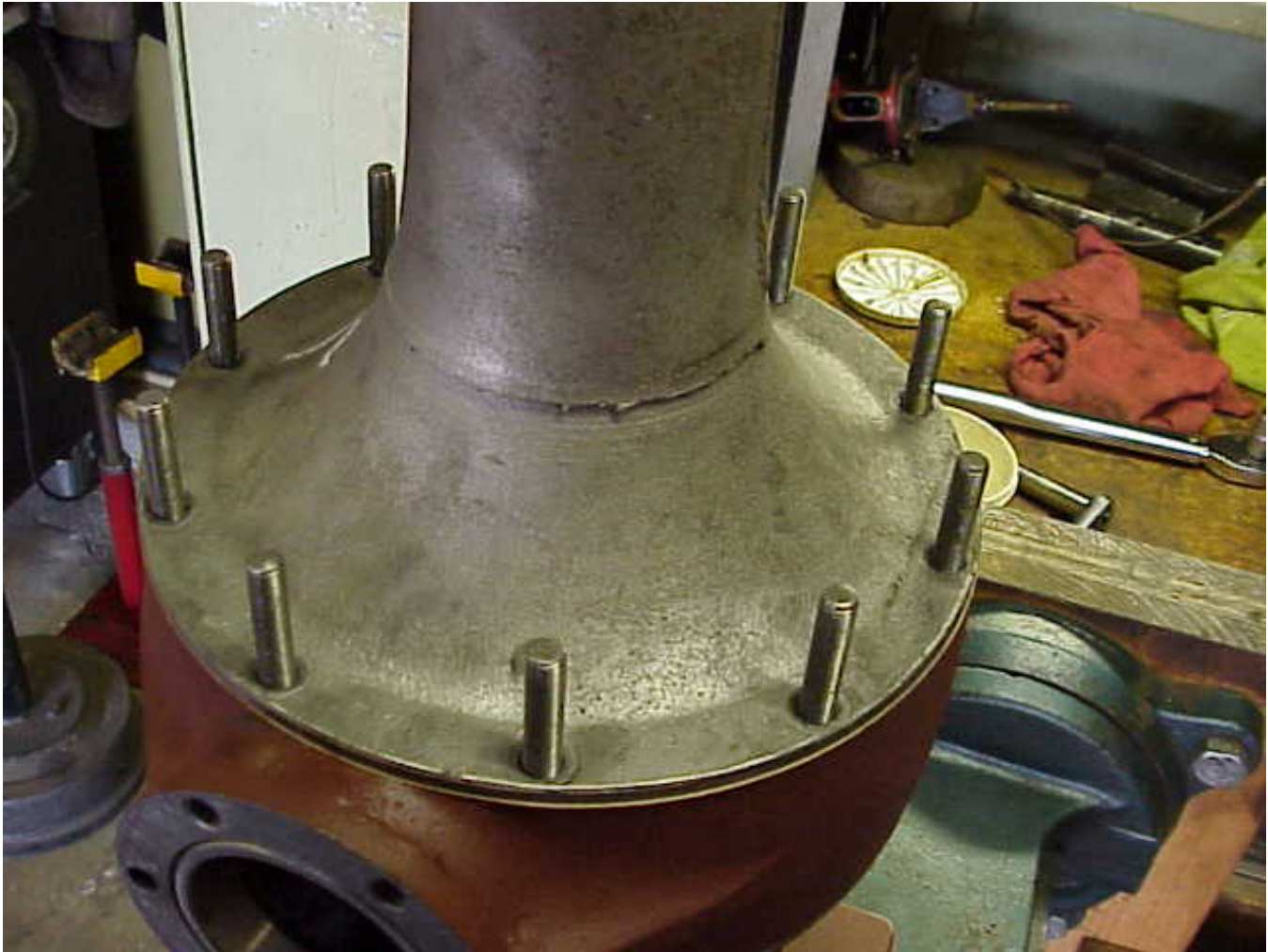
Photo P-30. The left axle housing is on top in the jig with alignment studs installed in the banjo: The studs will aid in the trial and error process of selecting the quantity and thickness of banjo gaskets required to set the pre-load.
