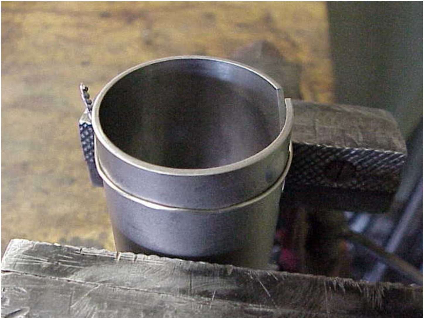
Photo P-48. Installation of torque tube roller bearing race: Squeeze the sleeve slightly in the vice to bring the split together. Wrap safety wire around it. Put a chalk mark on the top edge right above the dimple. Note dimple on the lower right side of the sleeve.
