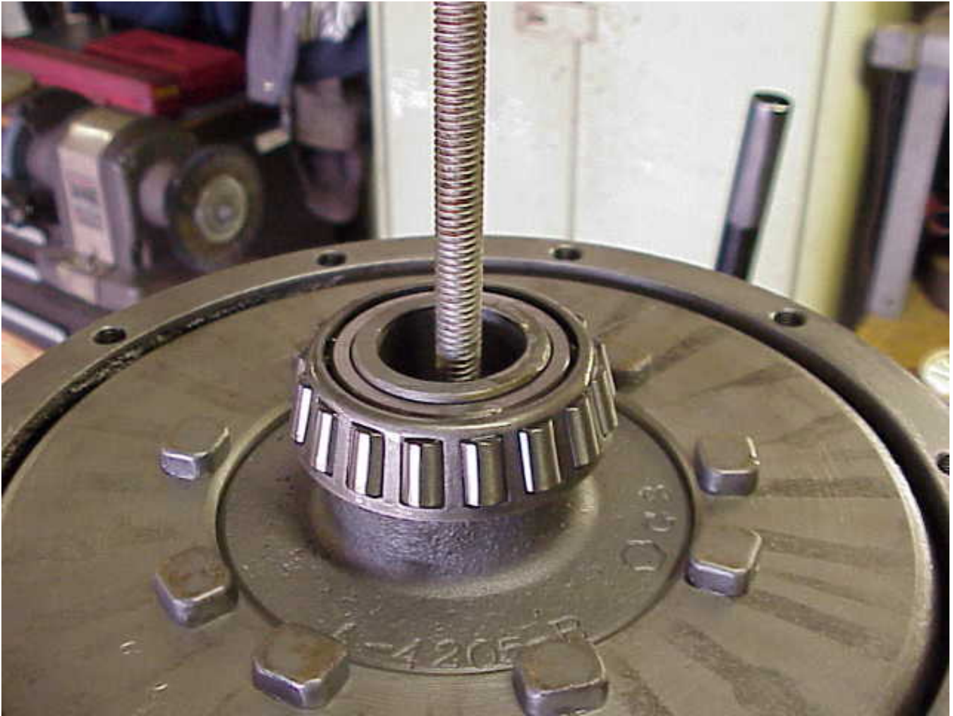
Photo P-33. The carrier pre-load measuring tool is inserted into carrier spider tool: The left axle housing has been removed to show that the pre-load tool shaft passes through the left axle housing and into the carrier where it threads into the modified spider gear yoke inserted between the two carrier halves. Turning the threaded shaft will rotate the entire carrier and ring gear assembly. The pre-load on the two bearings can then be read from a dial indicator torque wrench.
