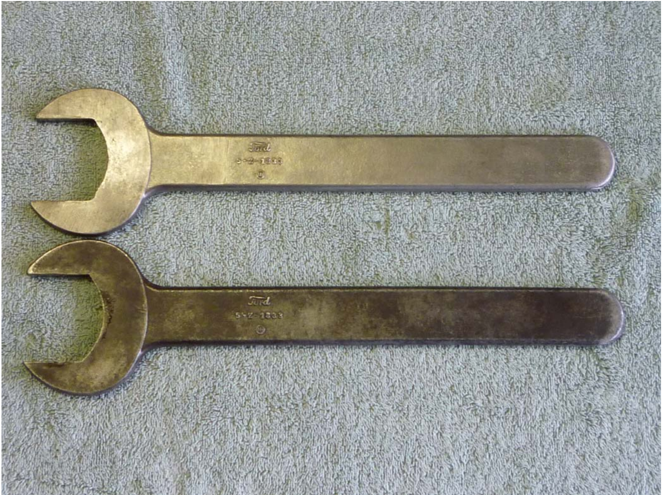
Ford factory wrenches used to set the pre-load on the later pinion gear assemblies that use the larger pinion nuts.
