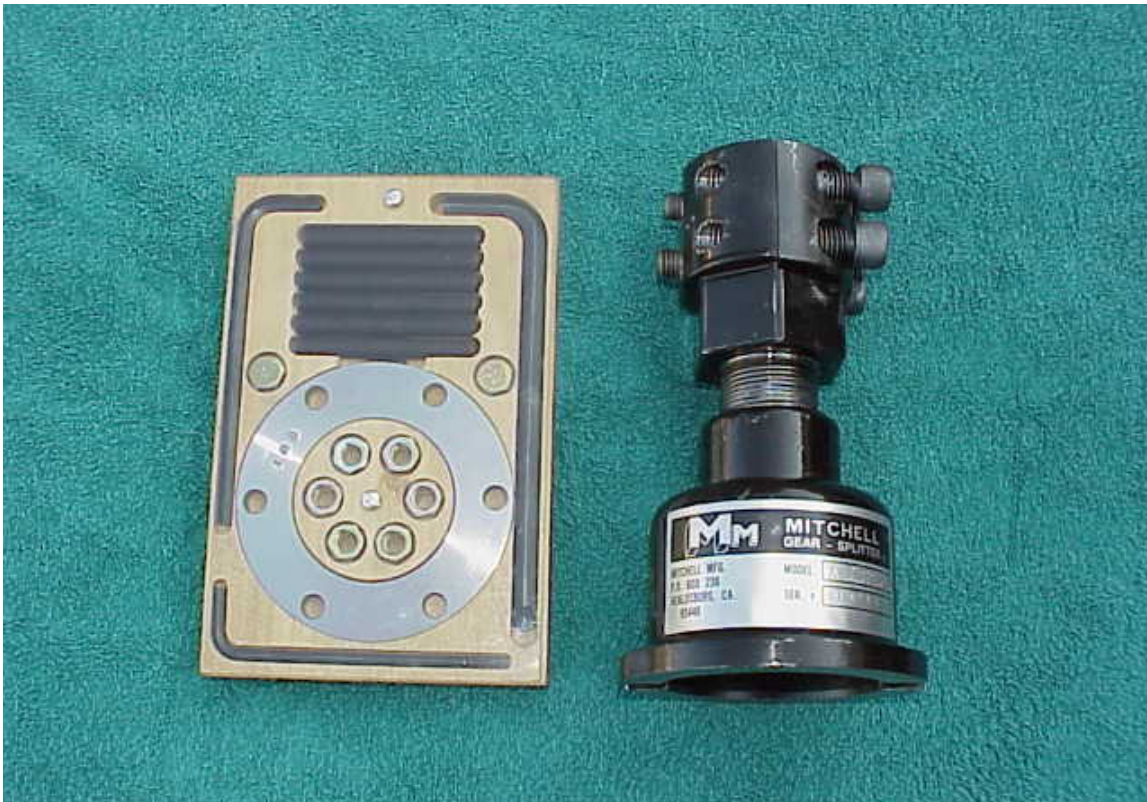
Photo P-2. Mitchell drive shaft puller tool: This tool can be purchased from the Mitchell Company. When purchasing an overdrive from them it can be rented.
