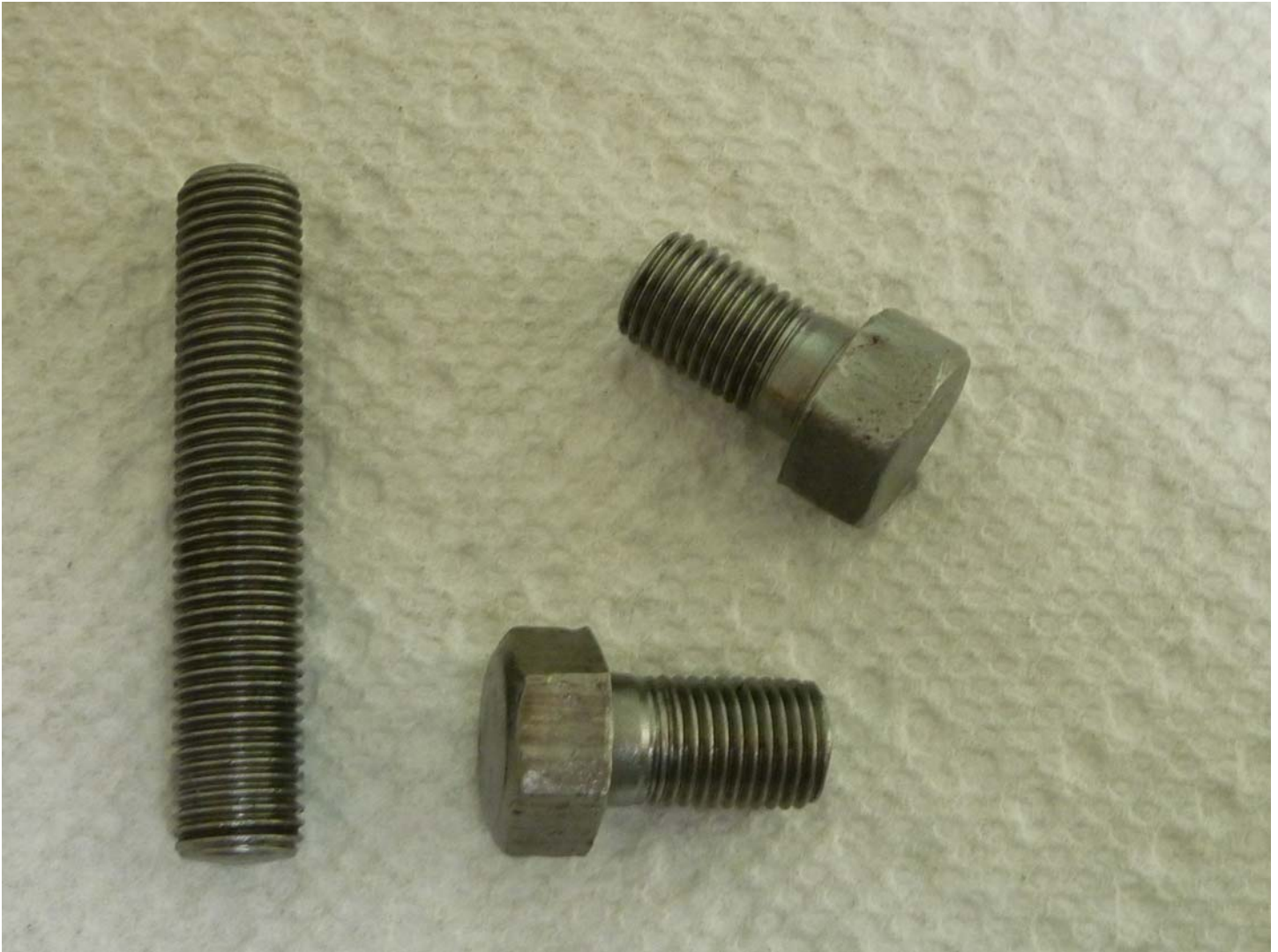
Photo P-17. Original banjo bolts, Quantity 20: Note space between the threads and the head of the bolt. Lock washers are not used with these bolts. The bolt head has a unique thickness. The stud at left is one of the alignment studs used to position the gaskets. The thread size is 3/8-24.
