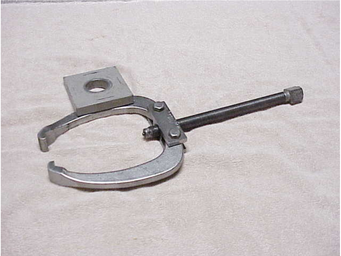
Photo P-4. Pinion gear puller tool: This tool was originally sold by Sears years ago. Its intended purpose was for the removal of the flywheel on small lawn mower engines. The block of steel with the hole was fabricated. A small bearing puller will also work.
