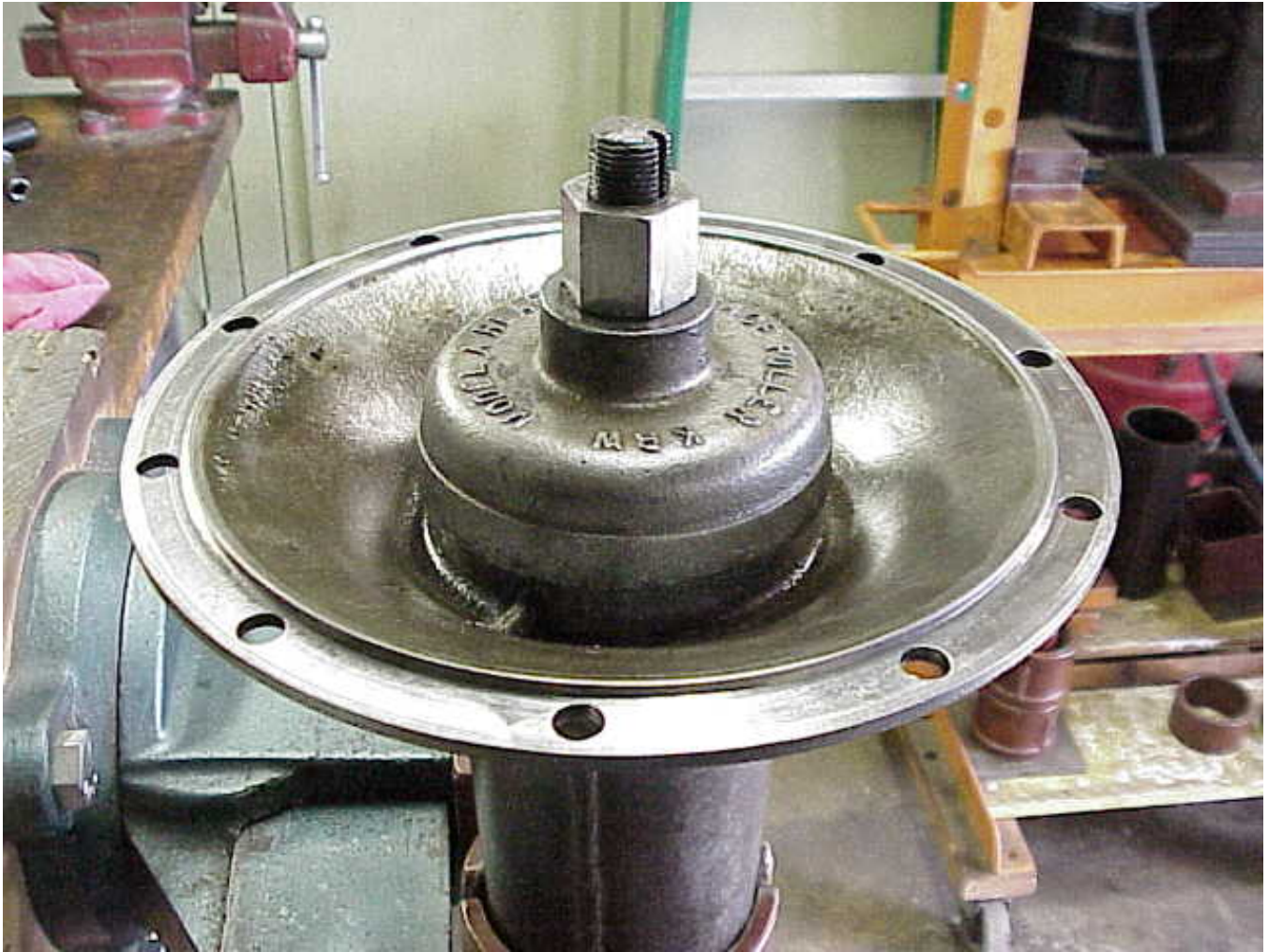
Photo P-10. Removal of axle housing bearing race: As the nut is tightened the race is removed. An impact wrench works very well for this task.
