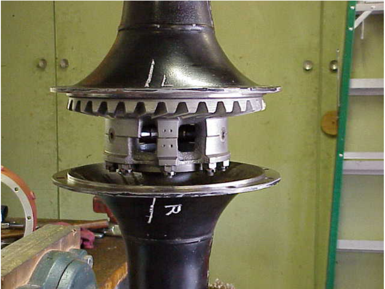
Photo P-32. Carrier pre-load adjustment: Add and subtract banjo gaskets on the left (top) side when the banjo is installed. Note the carrier half markers. These punch marks were in place when the rear axle assembly was taken apart. Center punch marks should not be made over the tunnel for any of the 9 carrier bolts as it will make it difficult to remove the bolt. Add the punch marks below and above the end of any of the three spider yokes.
