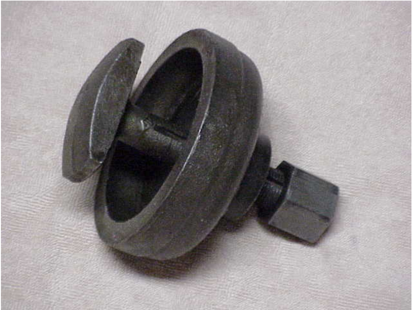
Photo P-9. K. R. Wilson axle housing race removal tool: The left end of the tool is placed down into the axle housing and grips the edge of the bearing race. As the nut is tightened it pulls the race out.
