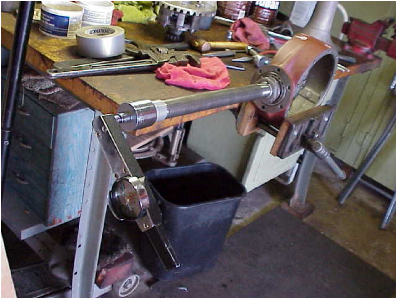
Photo P-43. Adjustment of pinion bearing pre-load: The adjustment of this pinion pre-load is being done with a Mitchell stub shaft installed. In this case duct tape was applied to the spline on the end of the shaft and a 36mm socket was pushed on over the end of the shaft. A 1&1\16" six-point socket is used over the end of a standard Model A drive shaft to set the pre-load.
