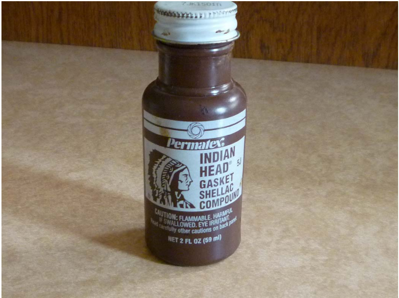
Photo P-47. Indian head gasket Shellac compound is recommended for use on the banjo gaskets. Coat each side of all gaskets used during final assembly.
