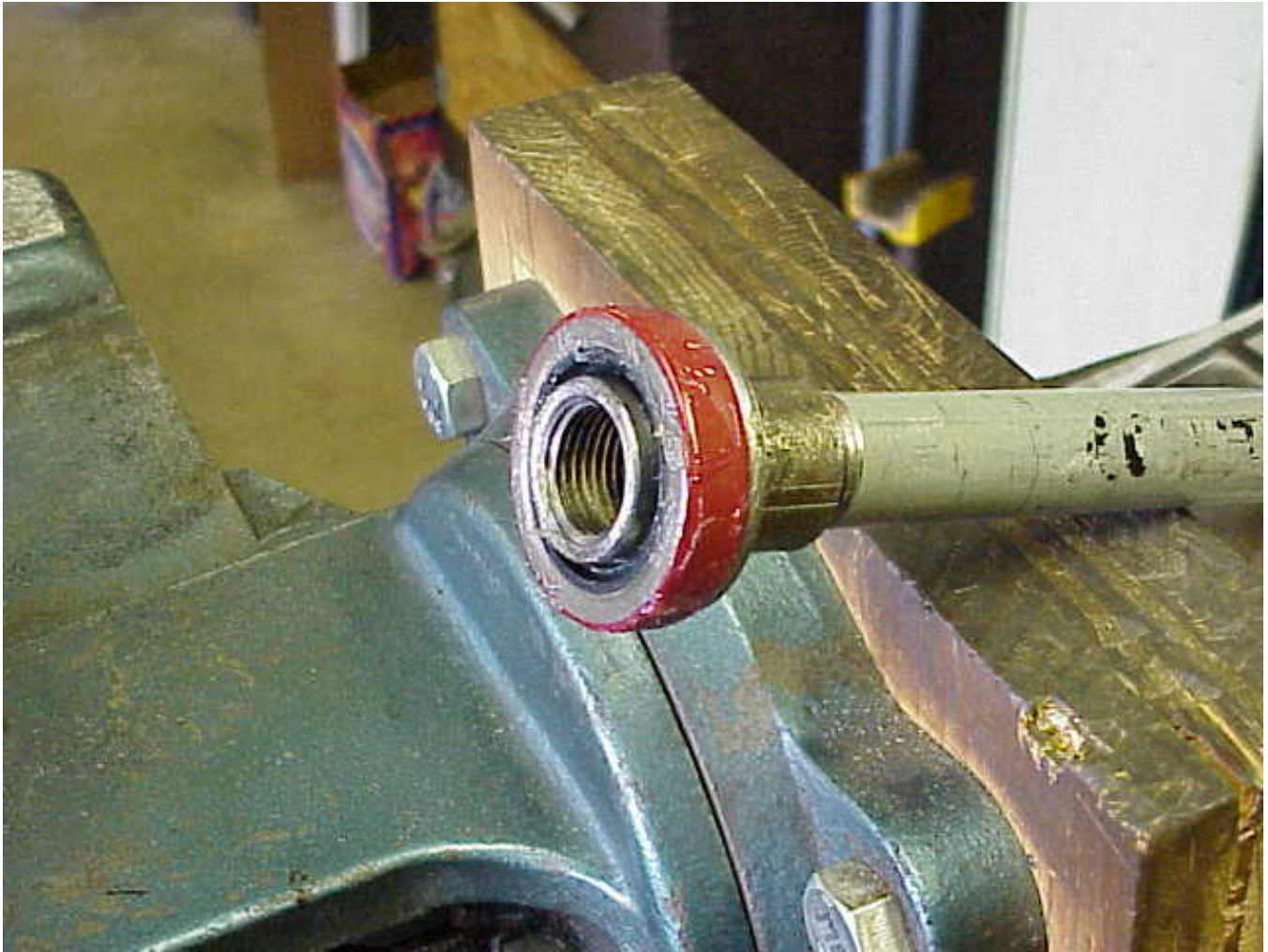
Photo P-25. The grease seal is inserted on the installation tool: Apply a coat of grease to the seal: The original grease seals were made by a company called Chicago Rawhide. They will have CR stamped on the side. The actual sealing portion of the seal was made of leather. New seals are made of neoprene.
