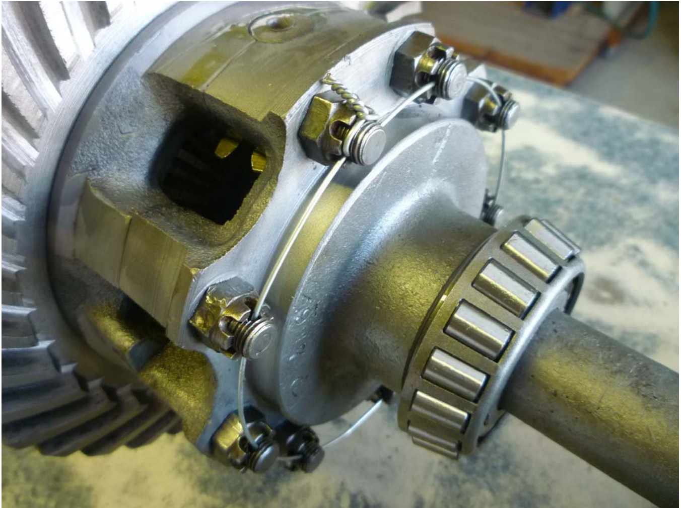
Photo P-46. The nine carrier bolts are torqued to 35 ft. lbs. and safety wired.
