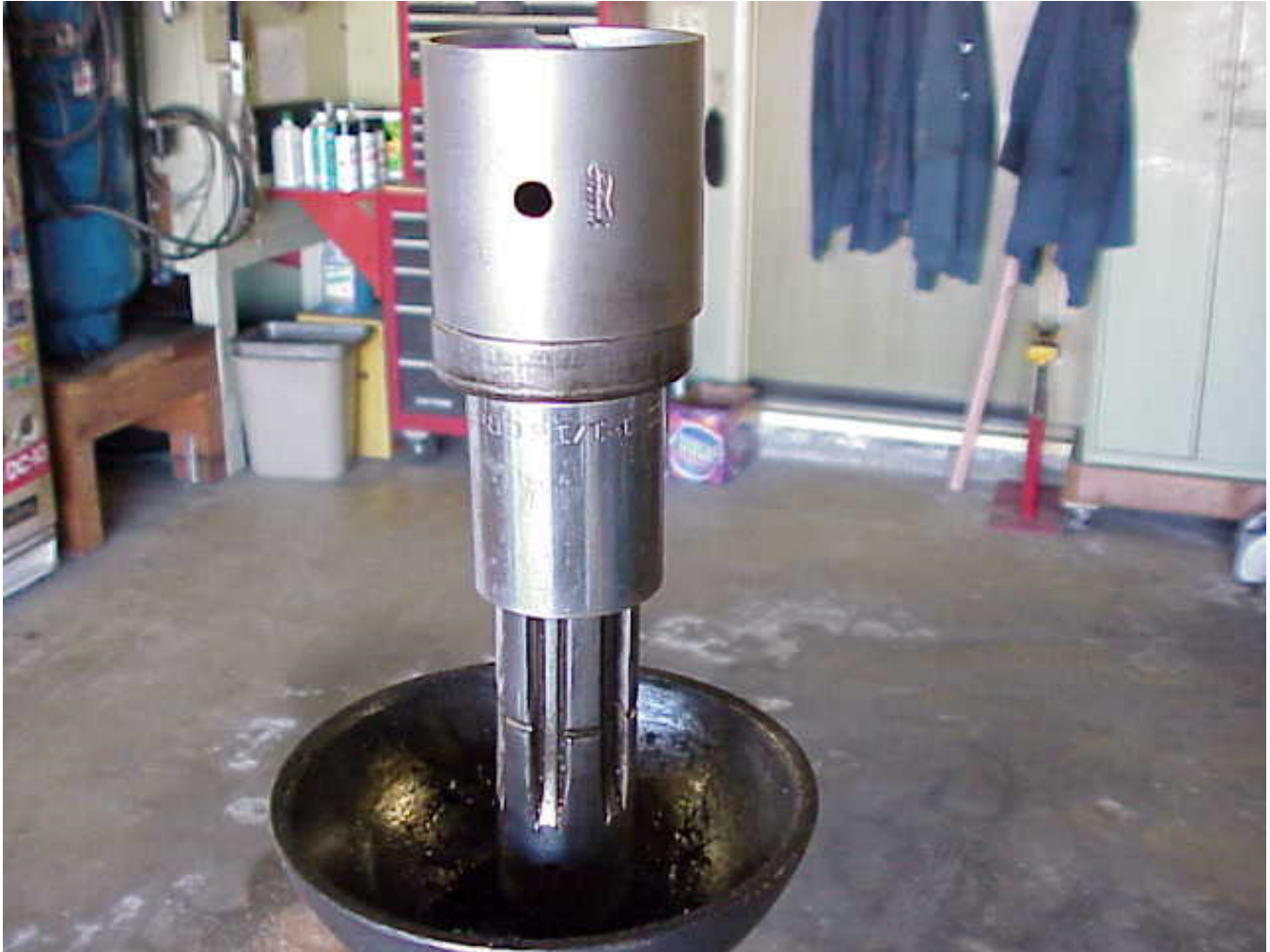
Photo P-1. Removal of the bearing sleeve and grease seal: The sleeve is at the top followed by the grease seal, then the socket. All are sitting on top of the drive shaft spline. A 1&1/16", 1/2" drive, six point socket fits over the splines on the end of the drive shaft.
