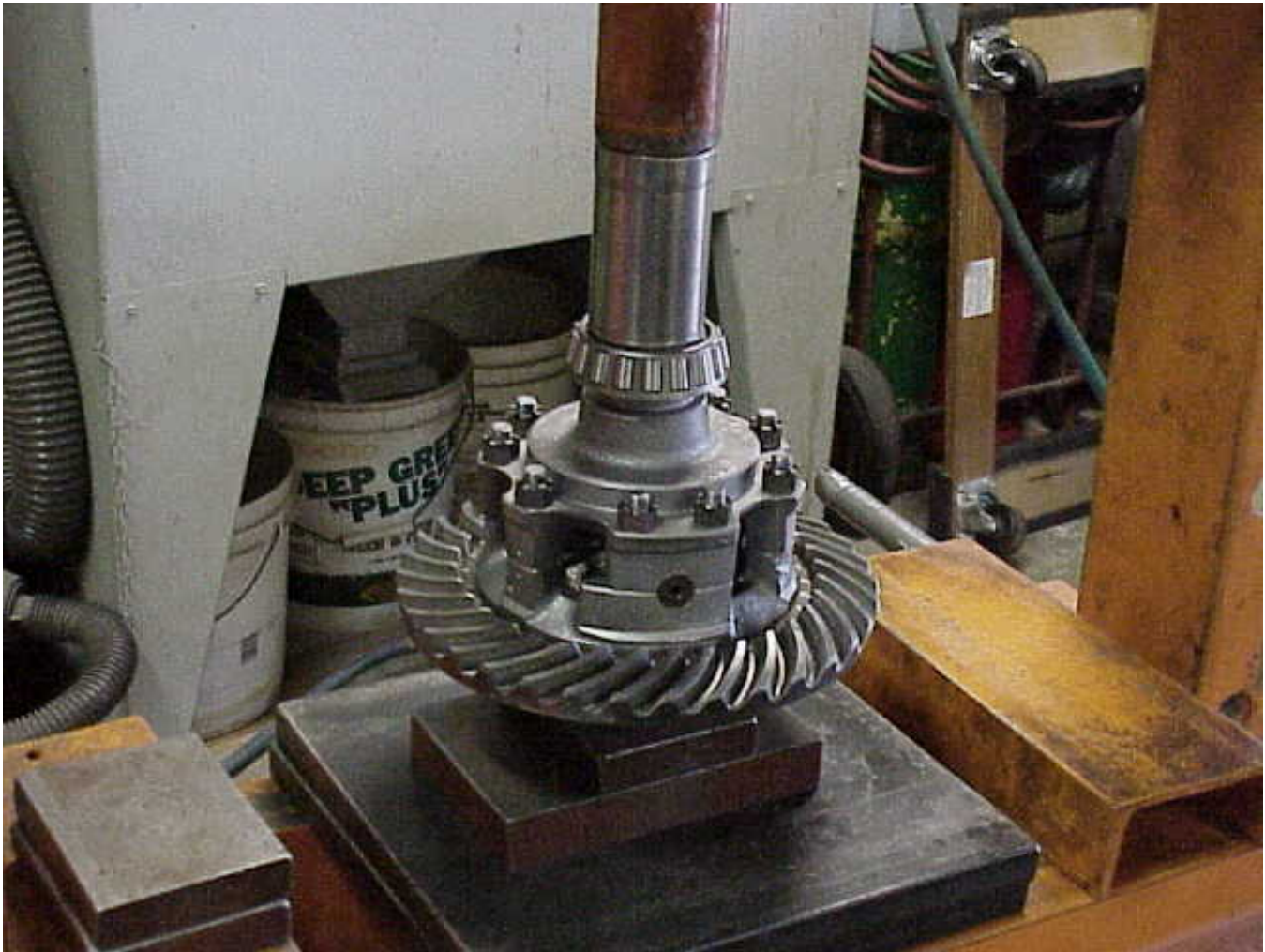
Photo P-19. Carrier bearing installation; New bearings are pressed onto the hub on each side of the carrier. They must press on with an interference press fit.
