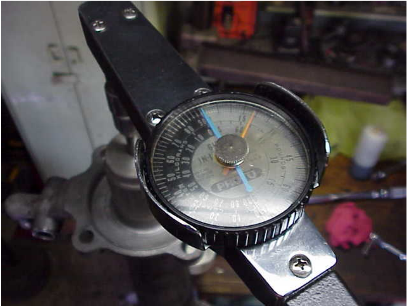
Photo P-35. Dial indicator reading 20 inch pounds of torque:
