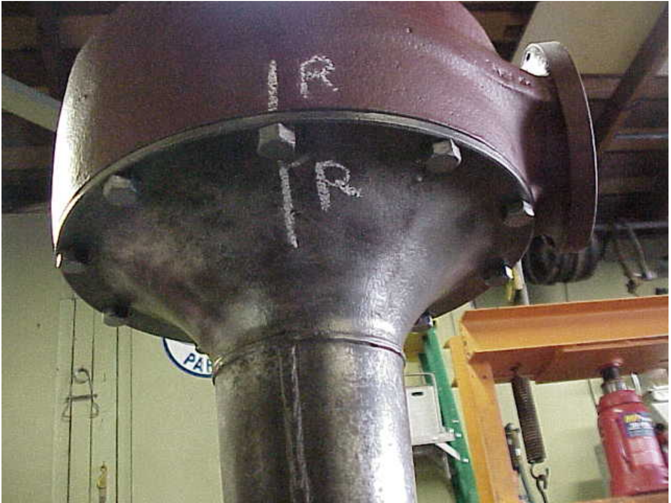
Photo P-28. The right axle housing is at the bottom of the jig: The banjo is on top and properly aligned with the mounting holes in the axle housing flange. It is recommended that the two axle housings and the banjo be marked for proper orientation before beginning the process.
