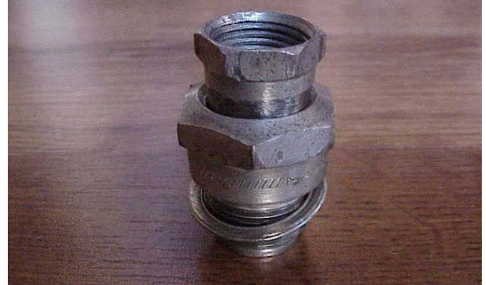
The modified base of a 3X spark plug and the adapter attached with 1/2"-20 threads.
