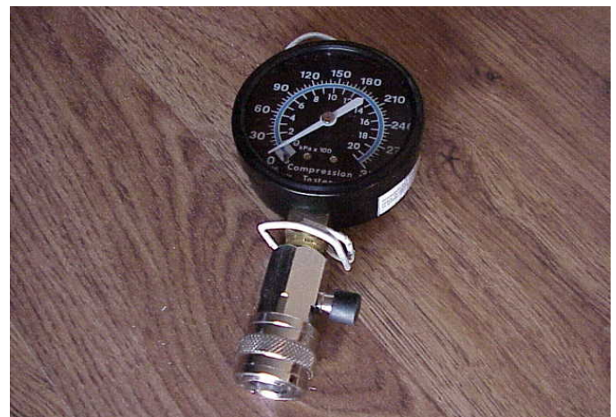
The gauge itself up close. A wire coat hanger allows it to be hung on the radiator support rods.
