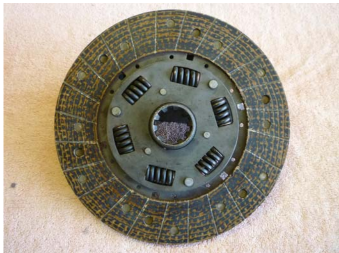
The six springs are not well secured. They can easily become dislodged.
