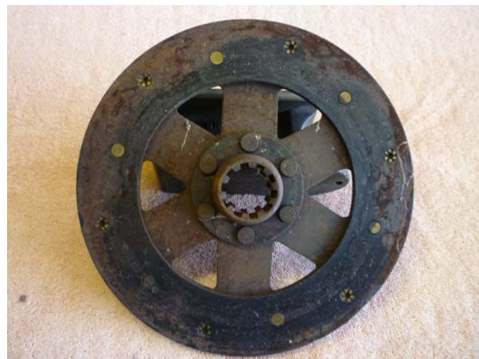
The original Model A clutch disk did not have springs.
