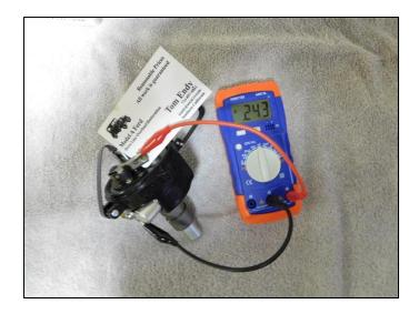
The Honeytek tester is a unique thing to have along on a tour. You can easily test a condenser while it is still attached to a distributor installed in a Model A. Simply remove the car's fuse, and slip a business card between the points. The plus lead of the tester is clipped to the arm of the points; the negative lead is clipped to ground on the distributor.
