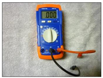
A Honeytek A6013L Capacitor Tester (called a condenser in automotive jargon) is available through Amazon for about \$17. The tester will tell you not only if the condenser is good or bad, but the actual value in micro-farads.
