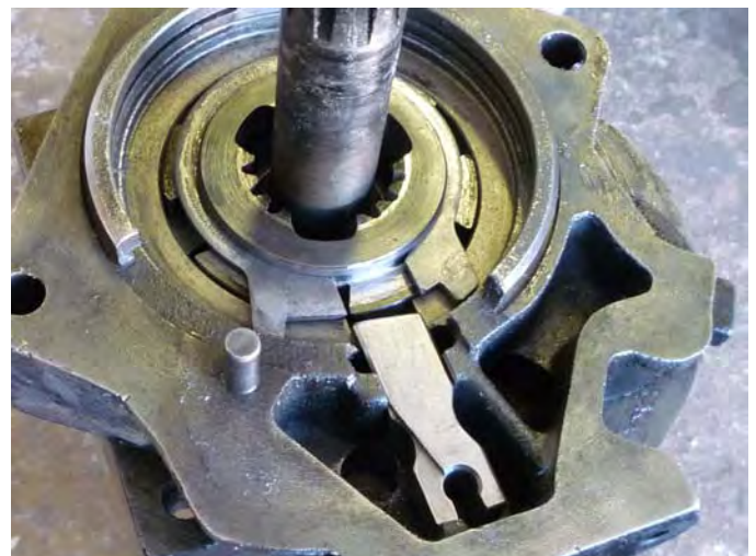
25. The pawl is installed with the machined relief at the lower left facing up. This will align the curve in the pawl with the hole in the casting. Note the direction of the angle at the top end of the pawl.
