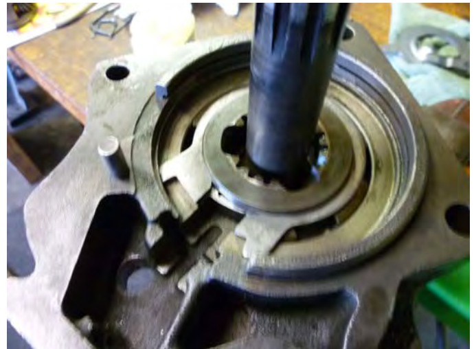
24. The blocking assembly is installed.
