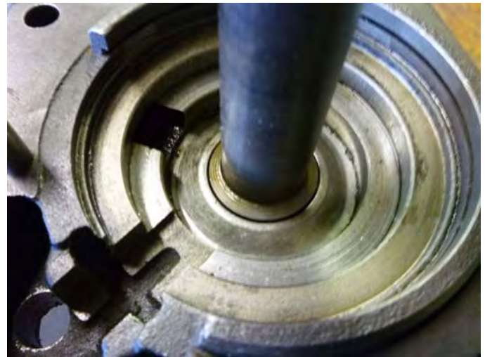
23. The blocking assembly is inserted into this recess. The pawl is inserted and actuates in the slot at lower left.
