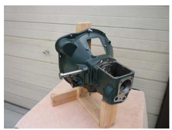
The positioning of the lag bolts and hex bolts are a nominal 3/4" from the sides and the centerlines. The only important consideration is that the lags in the counter sunk holes at the bottom of the base should be offset so as not to conflict with the hex bolts above.
