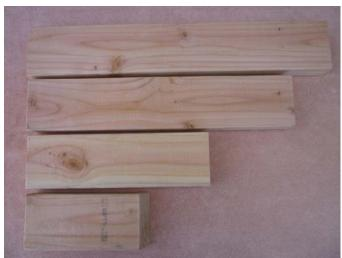
One ten-foot long 2X4 will make two stands with only a few inches of scrap left over. Four pieces for each work stand need to be cut to the following lengths. Top to bottom, 21", 18", 12", and 8". The 8" piece has one end cut at a 20 degree angle.
