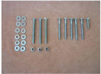
The hardware required is all  $5\16$ " with 1/2" hex heads in the following quantities. Three hex bolts 3&1/2" long, with three matching hex nuts, five lag bolts 3" long, one lag bolt 1&1/2" long, and twelve flat washers. The washers are 1/4", but will fit 5/16" bolts and lags.
