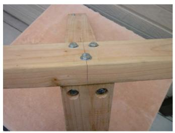
The base piece is secured from the bottom through the countersunk holes with lag bolts into the vertical piece. Care should be taken to offset the two holes so that the lags do not conflict with the two hex bolts above.
