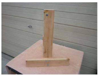
The cross piece is secured to the base piece with a lag bolt at the bottom. The two hex bolts above secure the vertical to the cross piece.
