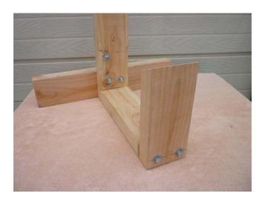
The 8" transmission support piece is attached to the rear of the base piece with two lags.
