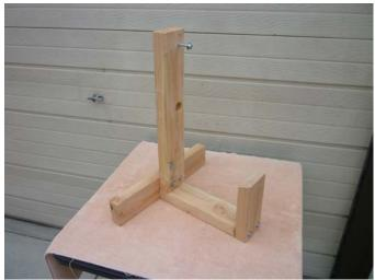
The vertical piece is 21" long. The cross piece is 18" long. The base piece is 12" long. The transmission support is 8" long with the top cut at a 20-degree angle and angle toward the front.
