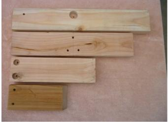
5/16" holes are drilled in each of the four pieces to accommodate the hex bolts and lag bolts. The 12"
