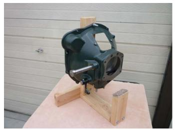
The work stand is constructed of 2X4's and provides a secure platform to remove and install parts on the bell housing. An additional support is added to the rear of the stand to allow the transmission to be bolted up to it.
